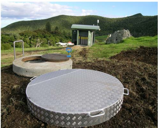
FIGURE 1: The seismic monitoring station at Lord Howe Island. In the foreground are the top of the seismic vault and vault cover with the hut containing the electronic processing equipment and battery bank in the background.
