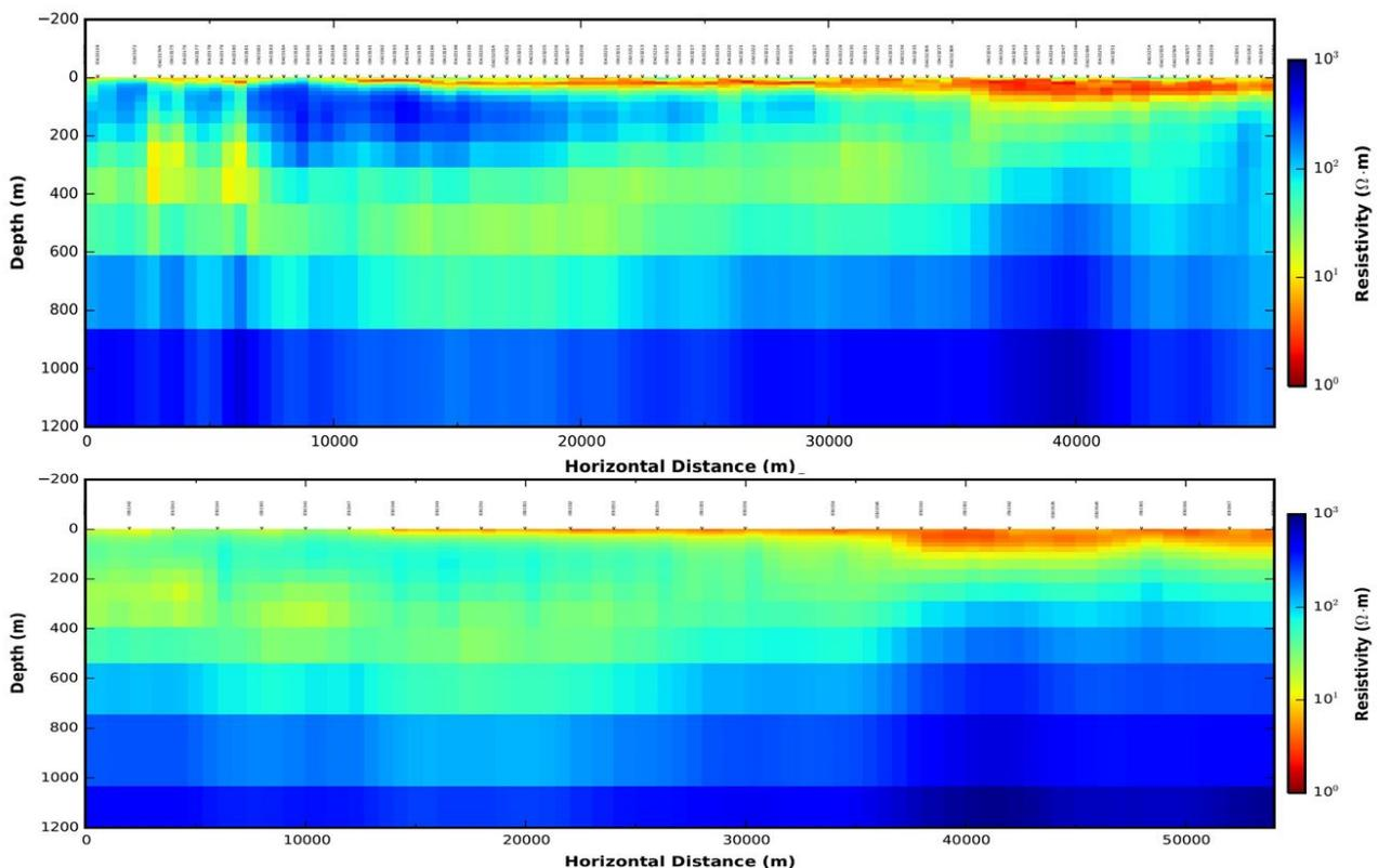
**Figure 4.** The top panel shows the result of inverting the AMT data for line 3000. The shallow low resistivity layer on the east of the section is interpreted as the Eromanga Basin sequence. The western end of the section shows the two-layer resistivity signature attributed to the Georgina Basin. The bottom section is the result of inverting the BBMT data on the same line. The two-layer resistivity of the Georgina Basin is subtle but present.
