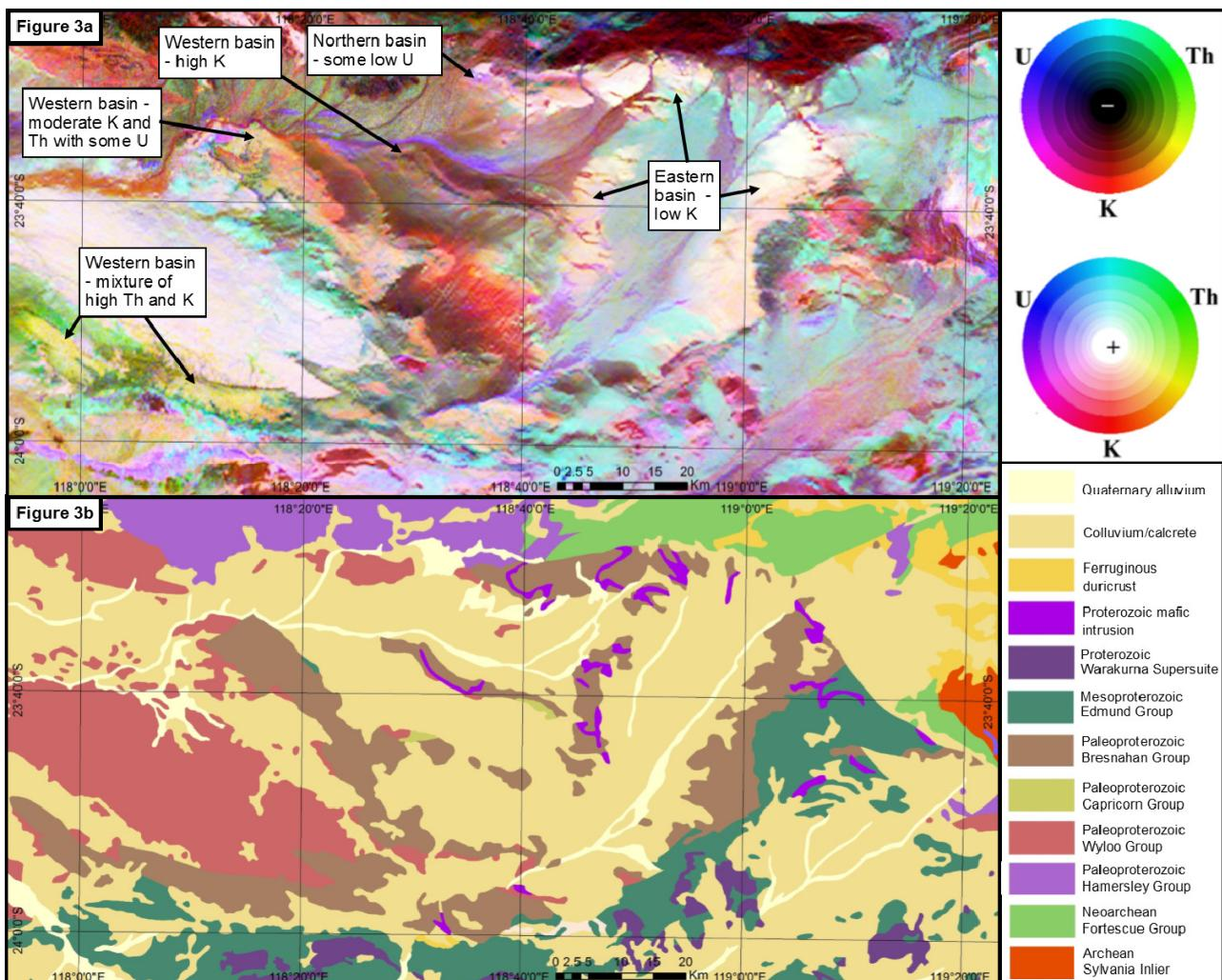
**Figure 3:** Highlights the radiogenic proportion differences across the basin, in particular the highly variable components in the western portion of the basin, Fig. 3a, a gamma ray coloured image showing the proportions of U, Th and radiogenic K, Fig. 3b, the surface geology for the region.
