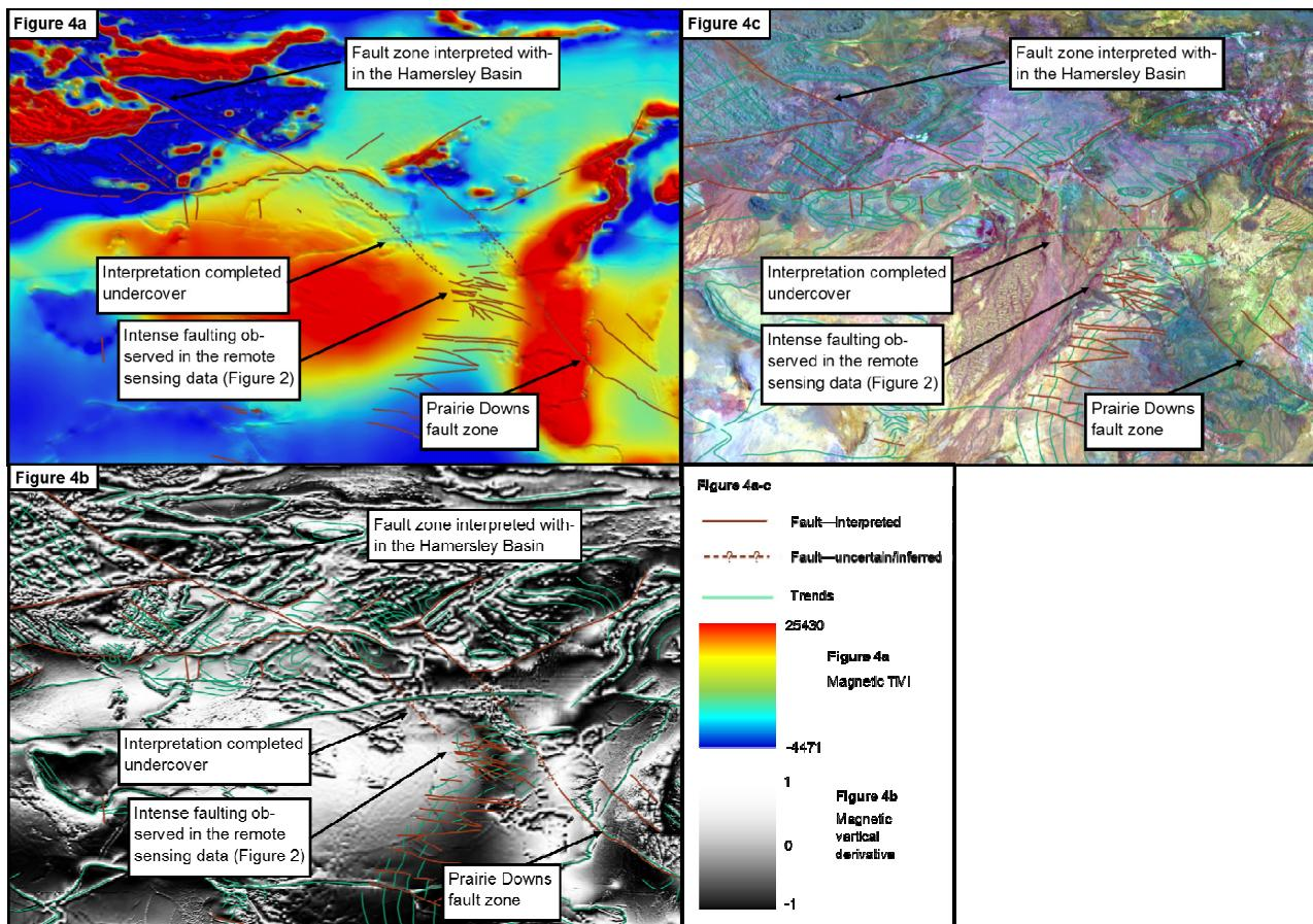
**Figure 4: Interpretation of a northwest-trending Prairie Downs fault, partly within or at the margin of the eastern portion of the Bresnahan Group. The orientation of the structure indicates a possible link with a fault interpreted in the older Hamersley Basin. Fig. 4a, Magnetic TMI, Fig. 4b, a processed vertical derivative of the magnetic data, Fig. 4c, Landsat 8 showing a 742 image.**
