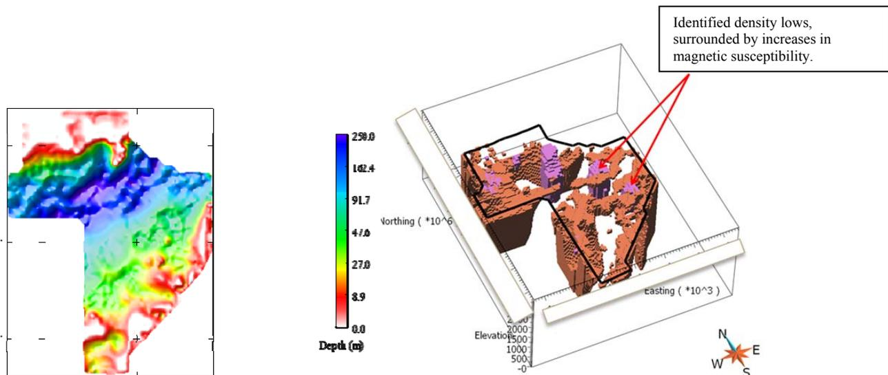
**Figure 6: Illustrates a map generated for the gravity survey extents of the final depth to basement topography incorporated in the constraining model (left). On the right, is a perspective view of domains queried from the inverted density and magnetic susceptibility models; density lows pink, magnetic highs brown. Evidence of possible alteration patterns around the identified density lows (red arrows).**
