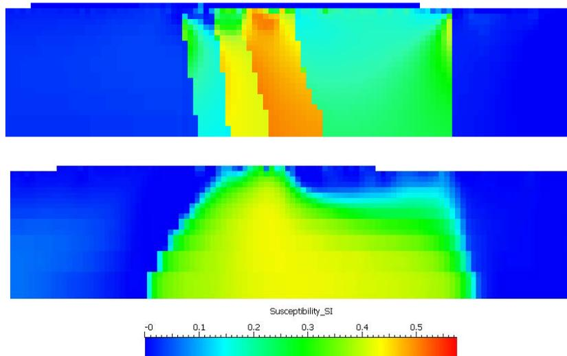
**Figure 4: Illustrates an E-W section (see Figure 3) of the geologically-based model (top) and an unconstrained inversion (bottom). The geologically-based approach results in more compact domains avoiding diffuse subsurface magnetic susceptibility variations.**
