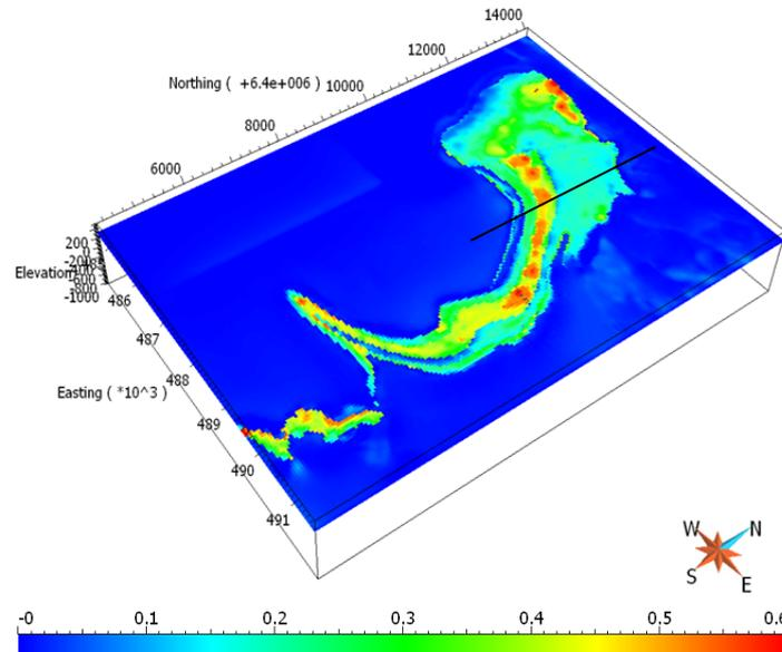
**Figure 3: Illustrates the final inverted model with 3D magnetic susceptibility variations within the domains. The black profile marks the location of the EW section shown below in Figure 4.**
