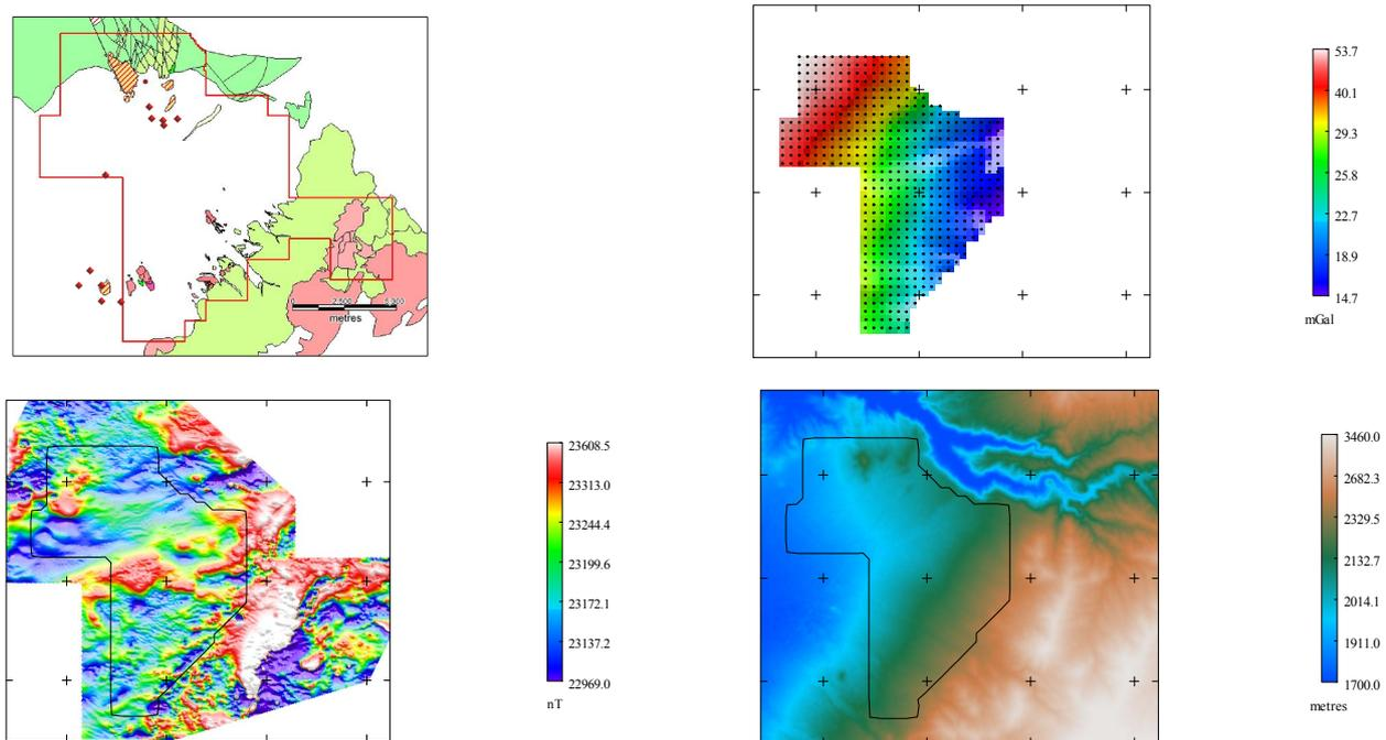
**Figure 5: Illustrates the key inputs for the integrated interpretation; (top left) geology mapping showing outcrop and drill hole locations (red diamonds), (top right) gravity, (bottom left) magnetics (TMI), (bottom right) topography.**
