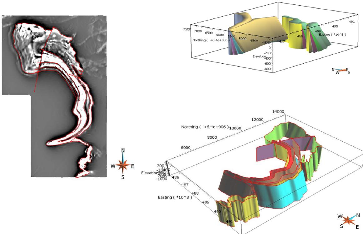
**Figure 1:** Illustrates the mechanics of interpreting the 3D magnetic domains; (left) interpreting sub-crop representation of domains, (top right) investigative modelling assessing various dips of domains used to compute magnetic responses for comparison with measured data and (bottom right) the collective wireframes from the investigative modelling used to construct a 3D geological model for the entire area for geologically constrained inversion.
