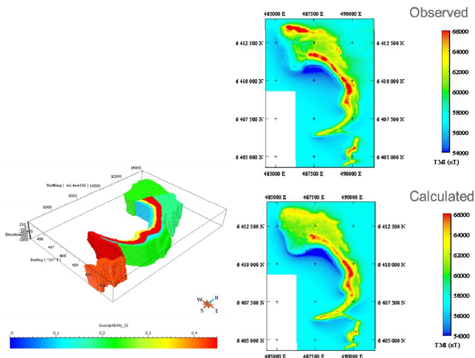
**Figure 2:** Illustrates the 3D magnetic domains coloured by magnetic susceptibility (left) in SI units and the measured and computed response of the final geological model attributed with homogeneous susceptibility.
