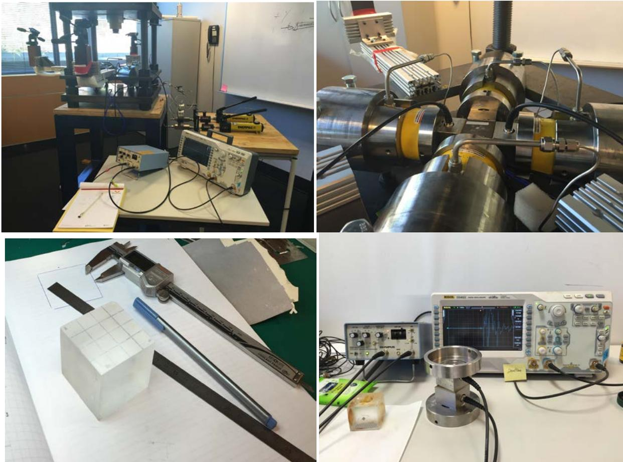
Figure 1: (a: top left) Setup of the experiment, (b: top right) 4 S wave transducers sealed on each actuators, (c: bottom left) PMMA sample polished and prepared to mount in the frame, and (d: bottom right) actuators dead time measurement
