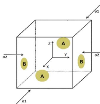
Figure2: Schematic showing the relevant geometry of the experiment and the orientation of transducers set up with regards to pressure direction.
