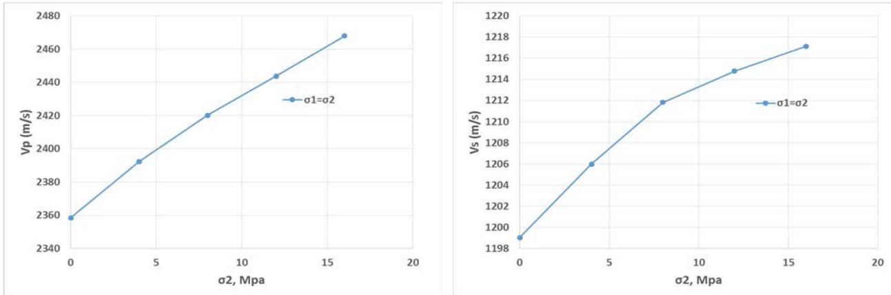
Figure 11:  $V_p$  and  $V_s$  on set A-A with increasing same stress in both axis
