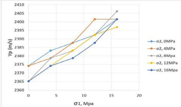
Figure 5: Vp on set A-A with the constant  $\sigma_2$  and increasing  $\sigma_1$
