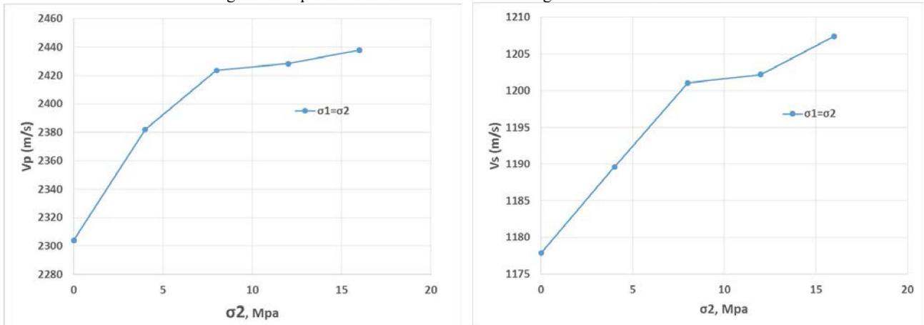
Figure 12:  $V_p$  and  $V_s$  on set B-B with increasing same stress in both axis
