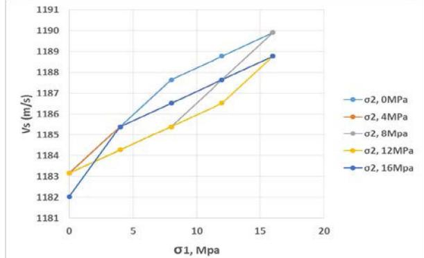
Figure 6: Vs on set A-A with the constant  $\sigma_2$  and increasing  $\sigma_1$
