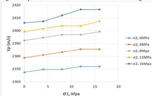
Figure 9: Vp on set B-B with the constant  $\sigma_2$  and increasing  $\sigma_1$
