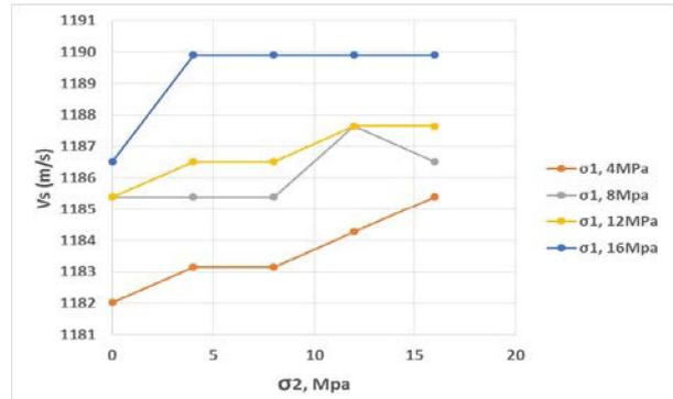
Figure 4: Vs on set A-A with the constant  $\sigma_1$  and increasing  $\sigma_2$
