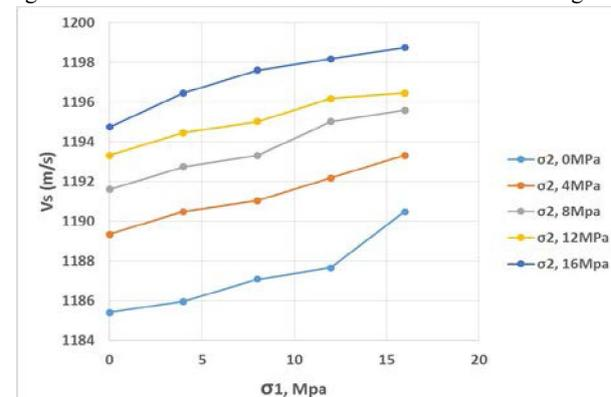
Figure 10: Vs on set B-B with the constant  $\sigma_2$  and increasing  $\sigma_1$
