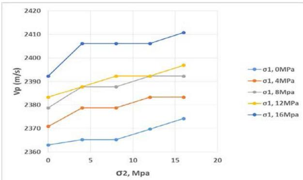
Figure 3: Vp on set A-A with the constant  $\sigma_1$  and increasing  $\sigma_2$
