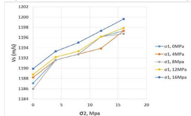
Figure 8: Vs on set B-B with the constant  $\sigma_1$  and increasing  $\sigma_2$
