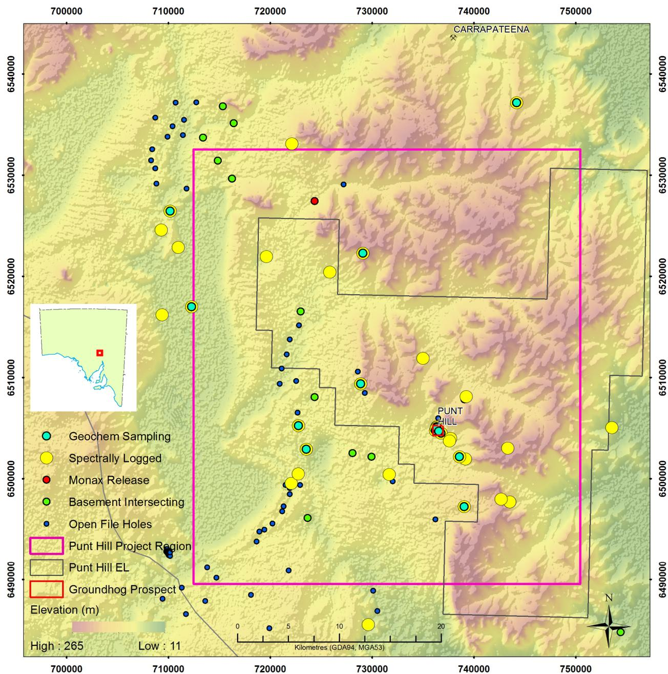
Figure 1: The Punt Hill study region, showing the location of the regional Punt Hill inversion (magenta rectangle), locations of drillholes sampled for the project and detailed Groundhog prospect inversion (red box). The digital elevation model (DEM) is in the background.
