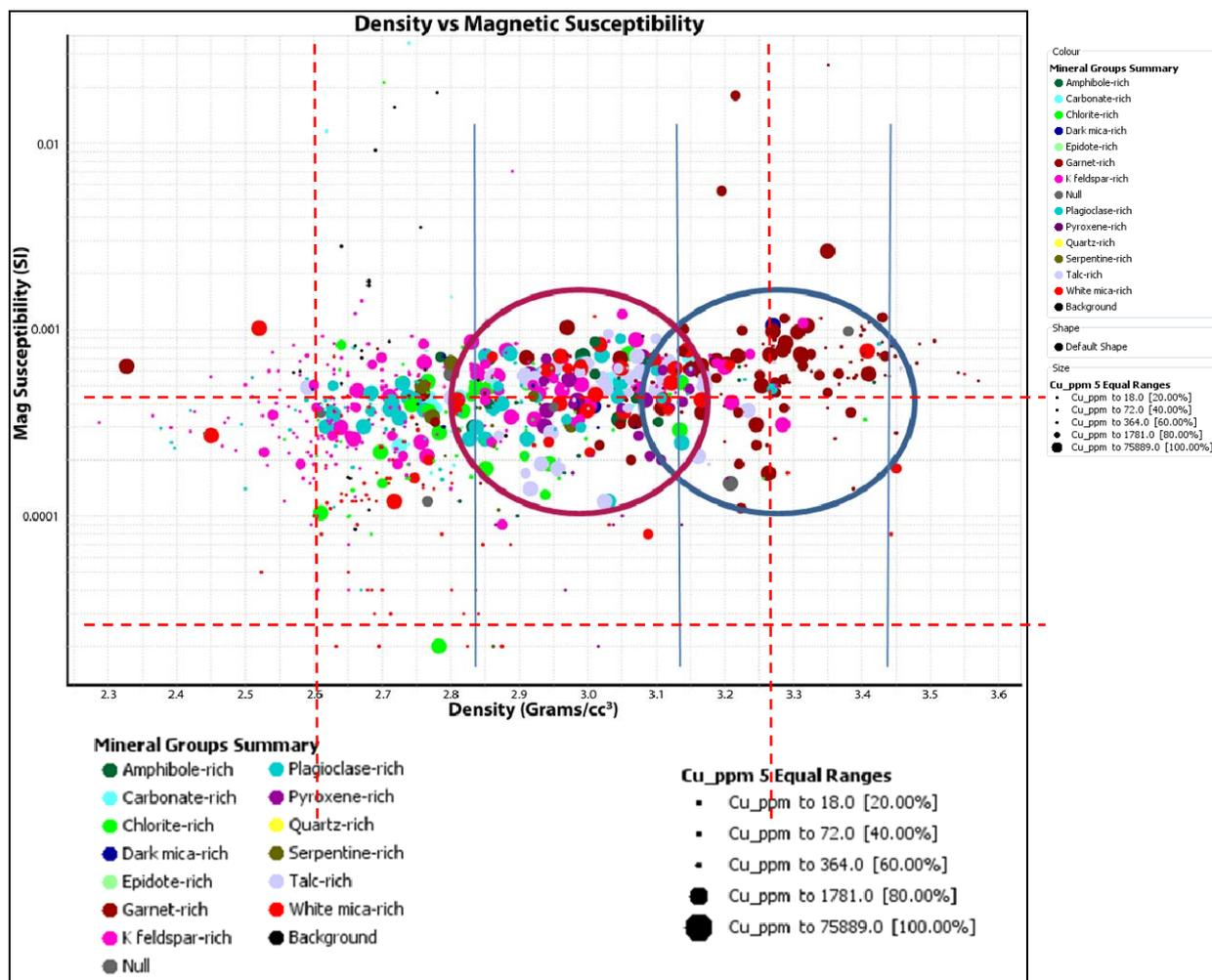
Figure 3. Mineral groups displayed by Cu ppm, density and magnetic susceptibility. At Punt Hill, prograde altered rocks have a moderately high density in the range of approximately 3.1 – 3.4 g/cc<sup>3</sup>. Retrograde overprinted rocks have a density range of approximately 2.8 – 3.1 g/cc<sup>3</sup>. Reasonable discrimination was observed between prograde and retrograde assemblages. Densities below 2.8 are considered to be background.
