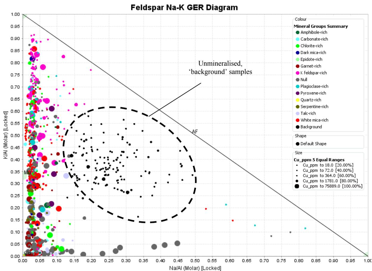
Figure 2. Feldspar GER diagram showing alteration assemblages derived from a combination of spectral and geochemical data. This plot of K/Al versus Na/Al values was used to define samples with minimal alteration. Alteration styles could then be associated with petrophysical measurements on the same sample.
