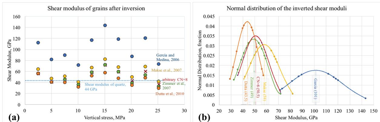
Figure-6: (a) Shear modulus of quartz grain after inversion using different coordination numbers. (b) Normal distribution of the inverted results.
