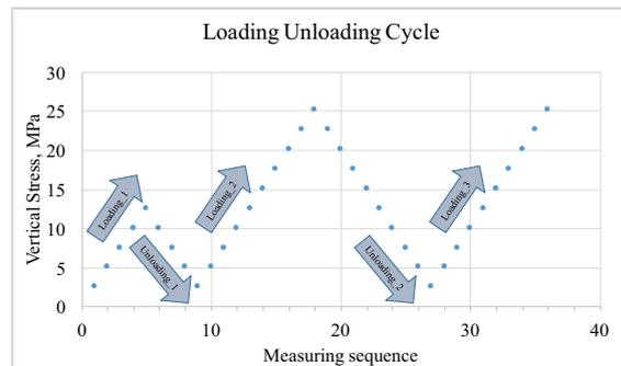
Figure-3: Loading-unloading procedure
