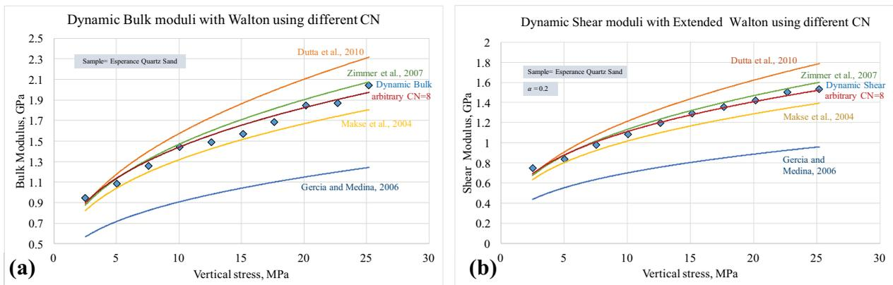
Figure-5: Dynamic elastic moduli of quartz sand pack with Walton model using different coordination numbers (a) dynamic bulk modulus (b) dynamic shear modulus.
