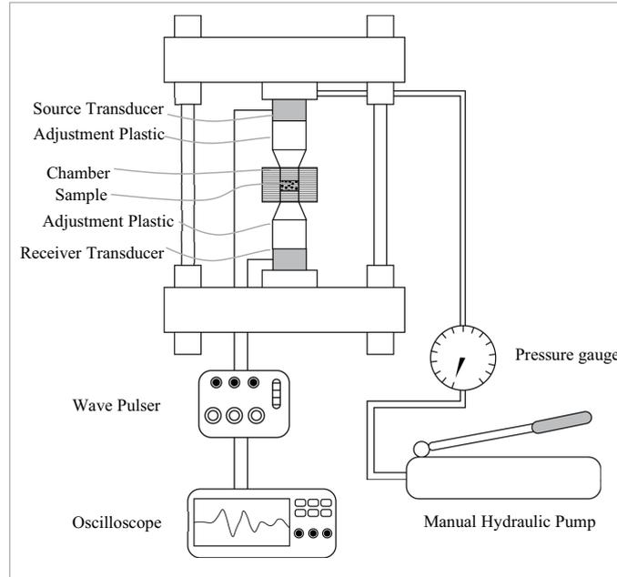
Figure-1: Basic equipment used in the experiment.
