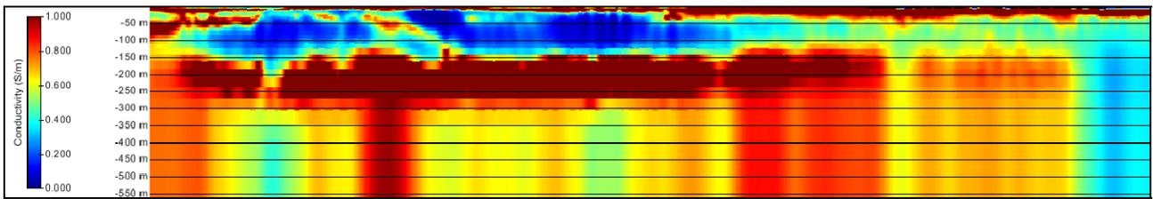
Figure 4. Most northerly AEM conductivity section (ENE-WSW) showing continuity offshore of fresh groundwater in the Point Springs Sandstone aquifer (dark blue). Fresh groundwater lenses are also preserved offshore in many of the AEM conductivity sections.
