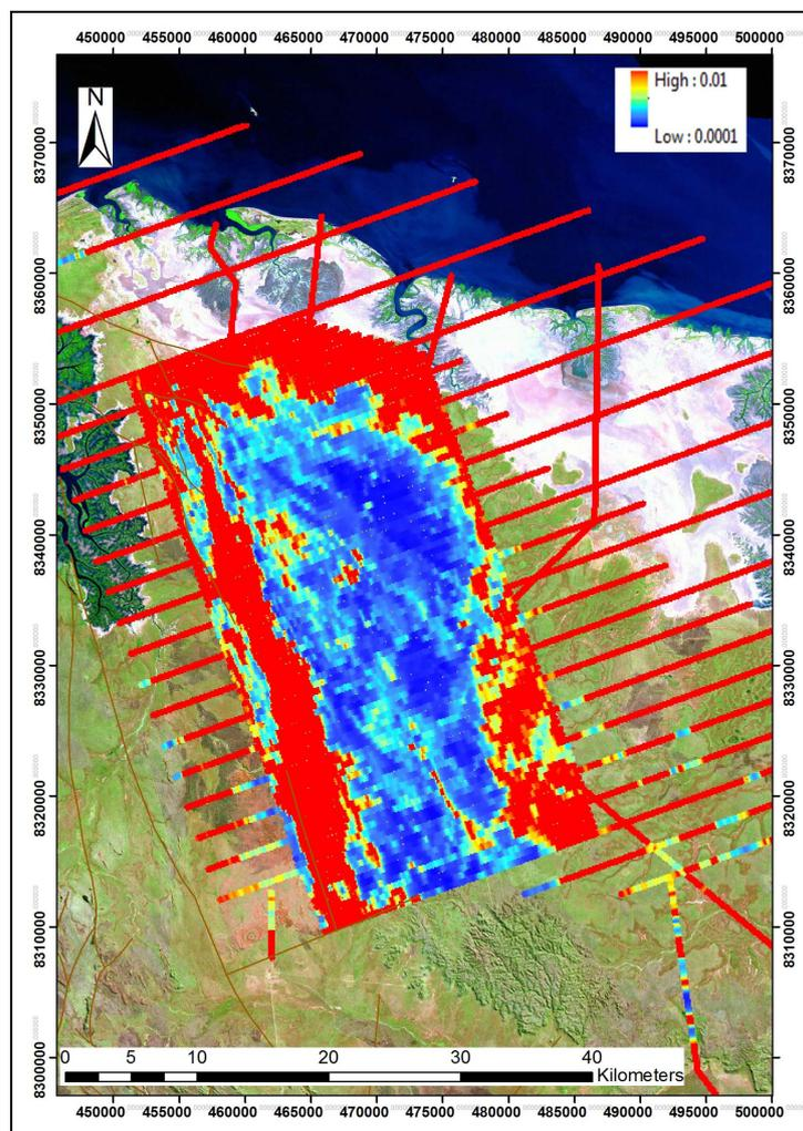
Figure 6. Conductivity depth slice (~30m) showing a window into the Point Springs Sandstone aquifer. The image has been colour-stretched to emphasise the more resistive areas (<0.01 S/m). The data show that the aquifer is resistive, but with subtle linear internal variations suggestive of faults. The eastern boundary shows the shallow seawater intrusion interface, while the western margin is interpreted to be bounded by a steeply-dipping fault-controlled shale unit.
