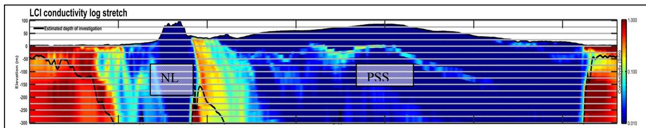
**Figure 3. Conductivity section oriented ENE-WSW showing the Ningbing Limestone and Point Springs Sandstone. The shallow seawater intrusion wedge is shown on the far right.**
