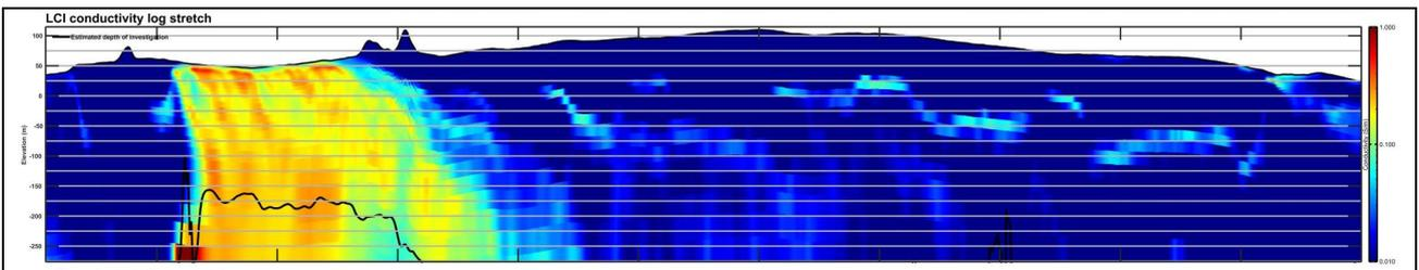
Figure 5. AEM conductivity section showing faulted shale layers within the Point Springs Sandstone aquifer.
