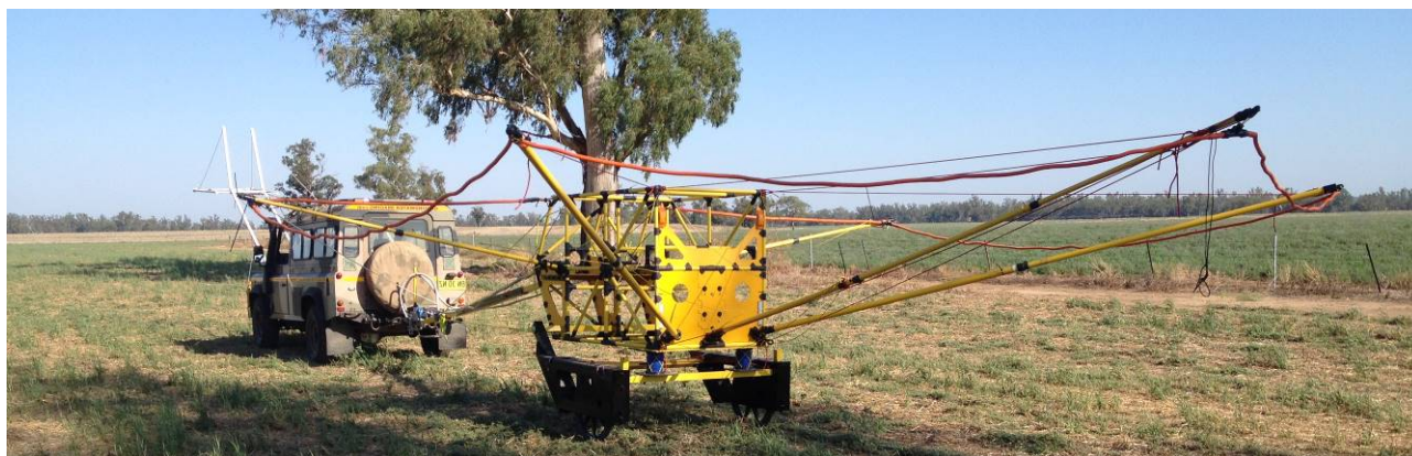
Figure 1: AgTEM 4 ™ cart with an additional receiver loop forward of the towing vehicle.
