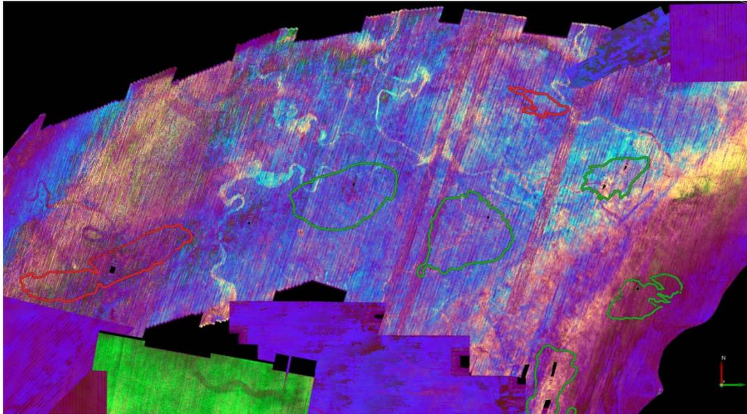
**Figure 1: An attribute blend at the bathymetric surface of the 3DGeo Gippsland MegaSurvey. The blue channel is Instantaneous Phase, the green channel Instantaneous Amplitude and the red channel is the standard signed seismic amplitude. Key petroleum fields are shown by red (gas) and green (oil) polygons. The Pleistocene drainage channel network shows good contrast with the surrounding alluvial plain.**
