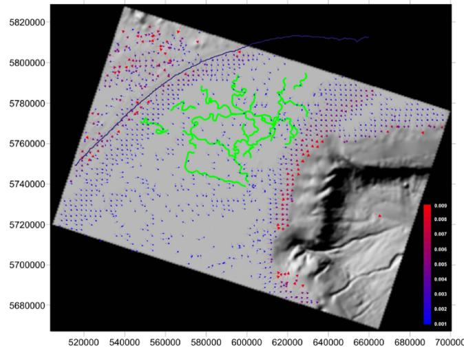
**Figure 2: Shaded relief image of Gippsland Basin bathymetry. Vectors show maximum surface gradients in the range 1-in-1000 to 9-in-1000 (the limit of natural rivers). Vectors are missing on the shelf where it is too flat to register, a band which coincides with the Pleistocene channels interpreted from 3D seismic data.**
