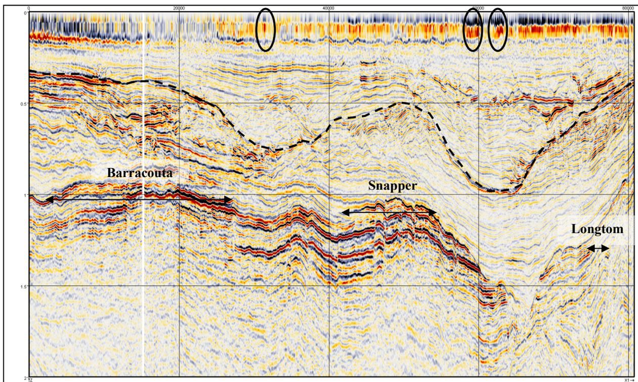
**Figure 3: An arbitrary line through the 3DGeo Gippsland MegaSurvey that links through Barracouta, Snapper and Longtom field areas. These fields sit within Latrobe Group reservoirs (high amplitude). Pleistocene channels are indicated by ovals highlighting signal amplification (high acoustic impedance contrast) and TWT push-down near the top of the section. The Mid-Miocene unconformity is shown by the dashed line.**
