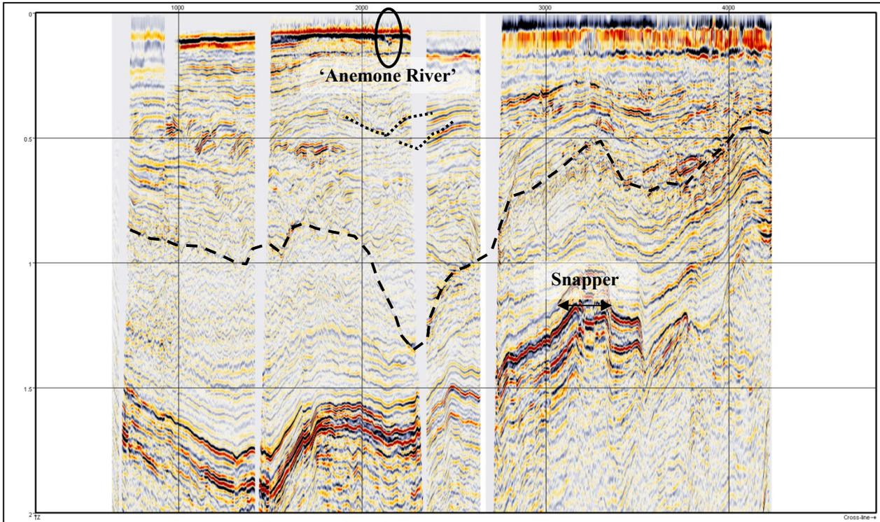
**Figure 4: Inline 2807 from the 3DGeo Gippsland MegaSurvey. The Snapper oilfield is shown. The ‘Anemone River’ is indicated by an oval highlighting TWT push-down near the top of the section. The Mid-Miocene unconformity is shown by the dashed line. Two pre-cursor canyon head surfaces are dotted in the same lateral vicinity as the modern ‘Anemone River’. All three channel forms overlie a sharp local trough in the Mid-Miocene unconformity surface.**
