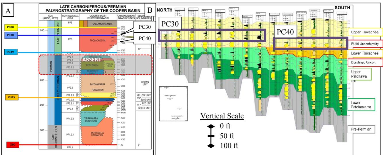
Figure 2: A) Stratigraphic section illustrating the Permian sequences in the Cooper Basin. B) North to South well cross-section highlighting the PC30 and PC40 reservoir targets.
