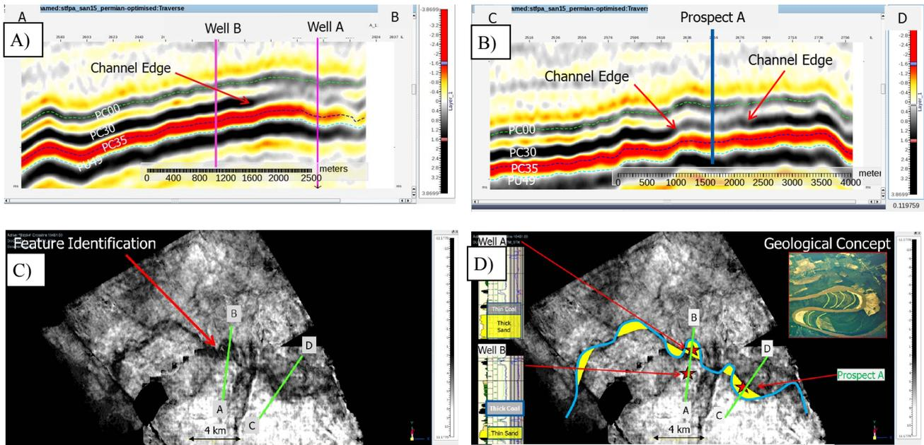
**Figure 3: PC30 feature identification screening process. A&B) Observation of seismic character change between well locations on arbitrary section lines. C) Identification of observed feature on seismic amplitude data. D) Integration of well and seismic data to develop a conceptual geological model.**
