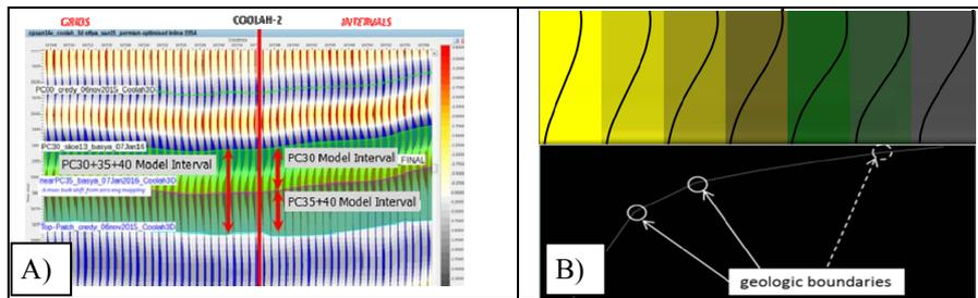
**Figure 4: A) waveform classification extraction intervals. B) Neuron classes identified for PC30 interval during process.**
