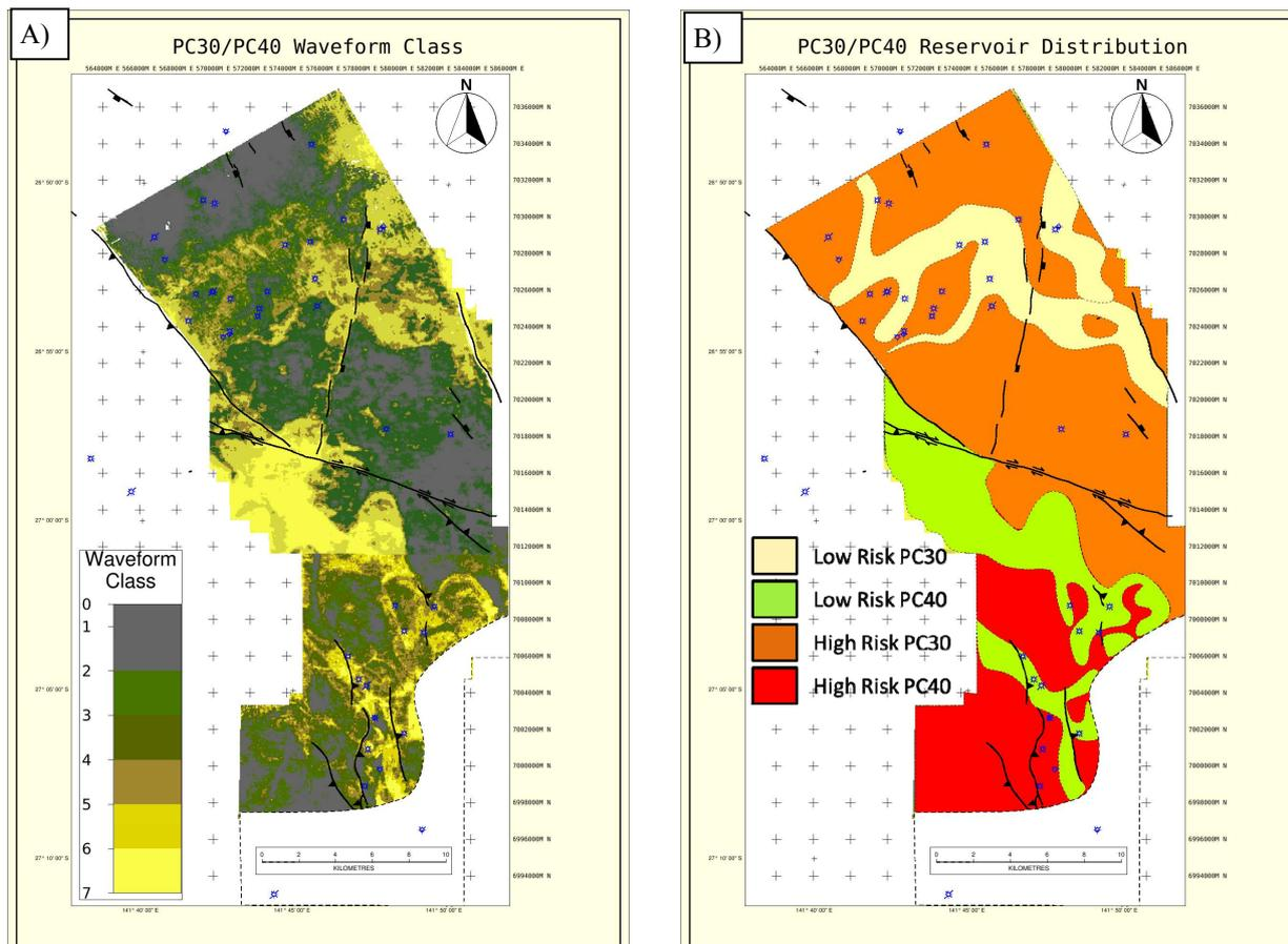
Figure 6: A) Waveform classification model for the three surveys. Risk of sand presence decreases with the higher class values. (Yellow = low risk reservoir, Grey = high risk reservoir). B) Reservoir distribution model and risk segment map incorporating the waveform classification model and well results.
