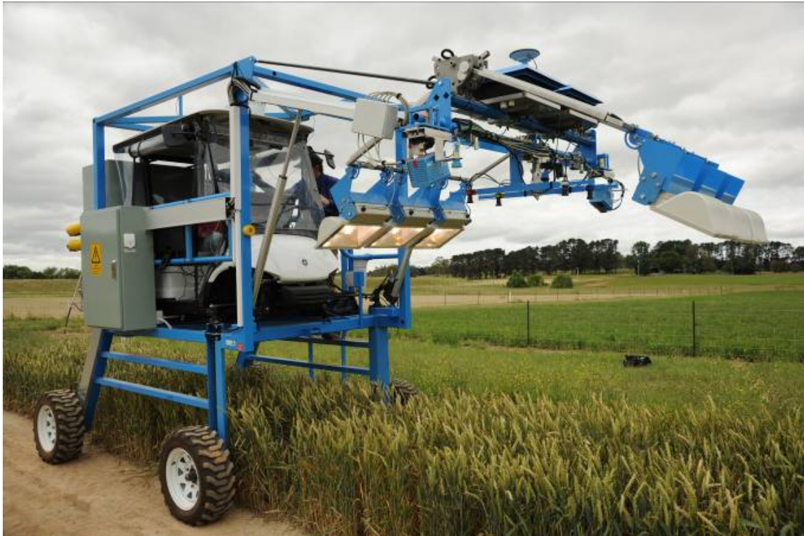
Fig. S3. Purpose built crop monitoring buggy fitted with: four RGB cameras for measurement of ground cover and plant establishment; LiDAR sensors to measure plant height and bio-volume; spectral radiometer from 300 to 2500 nm to measure NDVI and various spectral vegetation indices; three infra-red temperature sensors for crop canopy temperature.
