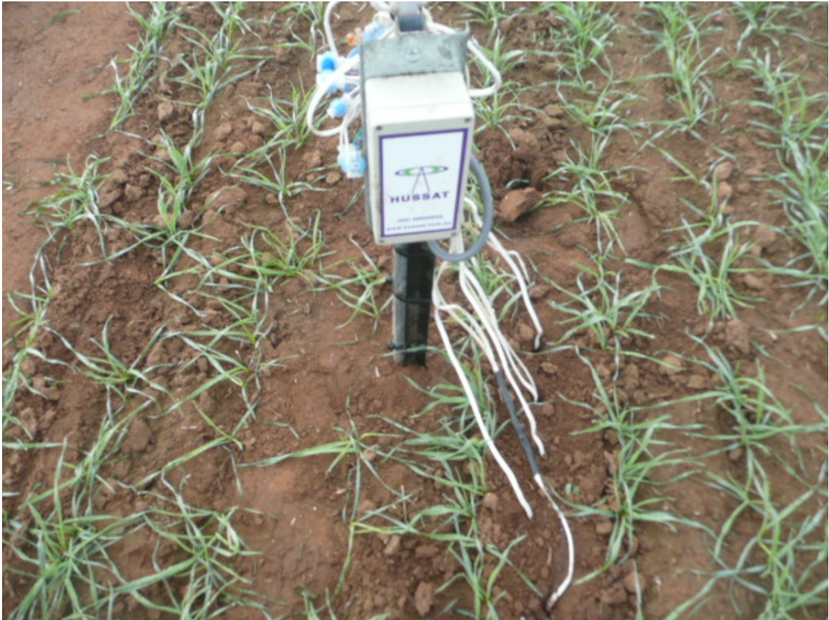
Fig. S1. Wireless data logger and radio transmitter for monitoring soil moisture and soil temperature at the Yanco MEF. Soil moisture status is monitored using gypsum block soil moisture sensors at six different depths (25, 50, 75, 100, 125 and 150 cm). Soil temperature is monitored using thermistors at two different depths (25 and 100 cm). Data is transmitted to a central base station located onsite and then transmitted very two hours via mobile phone network to the internet. Data is also stored locally on each logger for redundancy.
