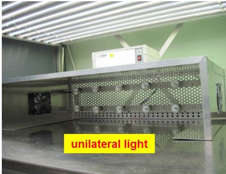
Fig. S1. The lateral light was produced by a halogen lamp in short-term light exposure experiment.
