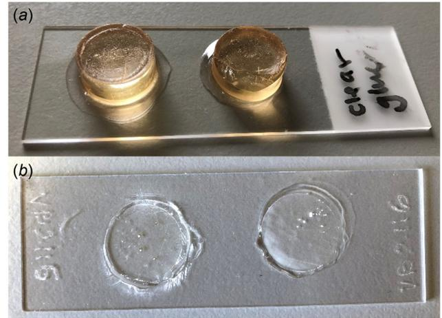
**Fig. 6.** Images of resin blocks with stylet sections when (a) glued to slide and (b) cut and polished.
