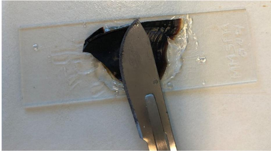
**Fig. 11.** Flattening beak half onto a slide with warm crystalbond adhesive.
