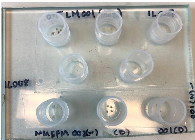
**Fig. 5.** Image displaying resin infiltration moulds used for stylet preparation including glass base, double-sided tape and plastic tubing.
