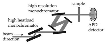
Fig. 1. Schematic of a typical set-up for nuclear forward scattering experiments. The incomming beam is reduced in bandwidth from  $\approx 300 \text{ eV}$  to several meV in two steps, scattered by the sample and detected by a fast avalanche photodiode detector (APD).
