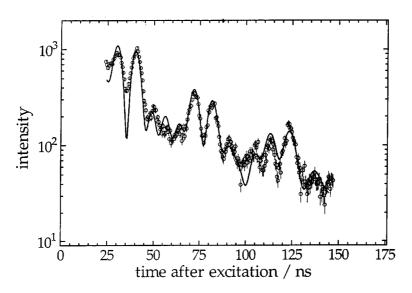
Fig. 2. Time evolution of nuclear forward scattering of synchrotron radiation measured with a 3  $\mu$ m <sup>57</sup>Fe foil at 15 GPa. The curve is an incoherent sum using the coherent time responses of  $\alpha$ -Fe (21%),  $\epsilon$ -Fe (38%) and the *coherent* sum of both (41%).
