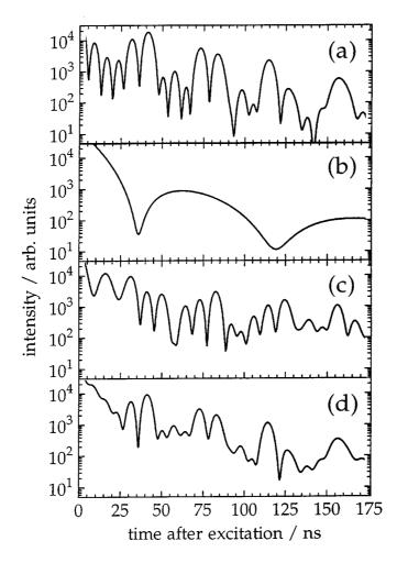
**Fig. 3.** Calculated time evolution of nuclear forward scattering of synchrotron radiation for  $(a) \alpha$ -Fe and  $(b) \epsilon$ -Fe. Also shown are (c) the coherent and (d) the incoherent sum of both time responses for 50%  $\alpha$ -Fe and 50%  $\epsilon$ -Fe.
