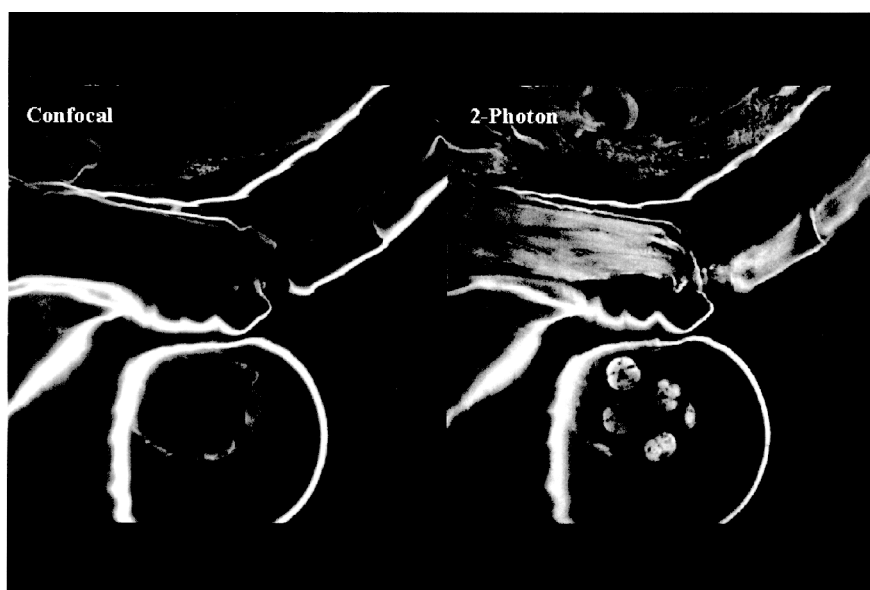
Fig. 7. Comparison of the confocal image (argon ion laser at 488 nm) and the two-photon image (Nd:YLF laser at 1047 nm) of the head region of an eosin stained Ceriodaphnia . The two-photon image shows significantly more detail at this depth into the sample.
