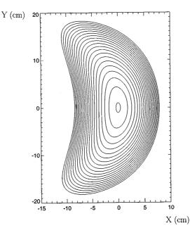
**Fig. 1.** Poloidal cross section of the H1-NF plasma at the plane  $\phi = 0$ . A (reduced) set of 21 nested magnetic surfaces is shown. The full equilibrium has been calculated with 100 magnetic surfaces equally spaced in the radial coordinate *s*. The position of the symmetry point  $\theta_0 = \zeta_0 = 0$  used in the numerical calculations corresponds to X = 7.6 cm and Y = 0 cm.
