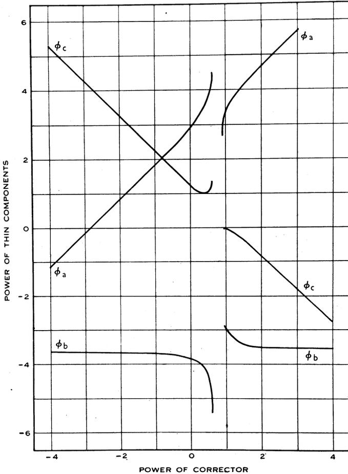
Fig. 2.—The curves show the dependence of the powers,  $\varphi_a$ ,  $\varphi_b$ ,  $\varphi_c$ , of the three thin components of a unit power triplet upon the parameter  $\chi$ . The useful range of  $\chi$ -values is seen to be approximately  $-2 < \chi < 0.4$ .
