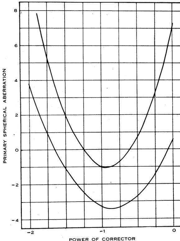
Fig. 8.—Curves showing the variation of the primary spherical aberration coefficient  $\sigma_1$  with the parameter  $\chi$  in unit power triplets from a given set of glasses. All other primary aberrations have been reduced to selected small values. The upper curve is for thin lenses and the lower curve for triplets with components of finite thicknesses.
