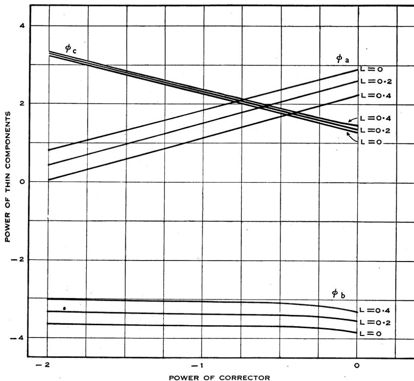
Fig. 6.—The effect of the variation of the axial chromatic aberration residual  $L$  upon the powers of the thin components is shown. A positive value of  $L$ , corresponding to a correction of longitudinal colour at an outer zone of the aperture, reduces the total curvatures in the first two components, but increases the power of the rear positive lens slightly.
