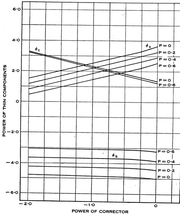
Fig. 4.—The graphs show the effect of the variation of the Petzval residual  $P$  upon the powers,  $\phi_a$ ,  $\phi_b$ ,  $\phi_c$ , of the thin components of a unit power triplet. Increase of  $P$  reduces the absolute values of the powers of lenses  $a$  and  $b$ , but has little effect upon that of lens  $c$ .
