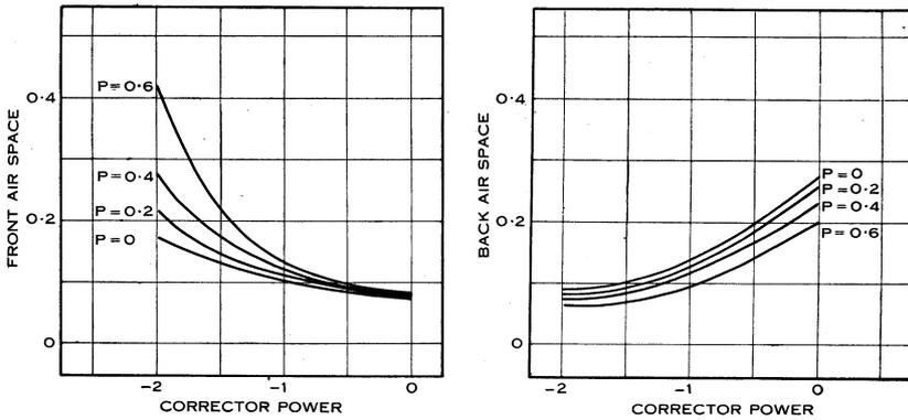
Fig. 5.—The corresponding effect upon the airspaces accompanying variation of the Petzval residual  $P$  is shown. An increase in the value of  $P$  enlarges the front airspace, particularly for large negative values of  $\chi$ , and diminishes the back airspace. For values of  $\chi$  near zero it is the rear airspace that is mainly affected.
