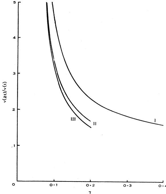
Fig. 8.—Values of  $v(2t)/v(t)$  at the centre of a solid with zero initial temperature and constant surface temperature as a function of  $T = \kappa t/a^2$ . Curve I: a slab; curve II: a cylinder; curve III: a finite cylinder whose length is equal to its diameter.
