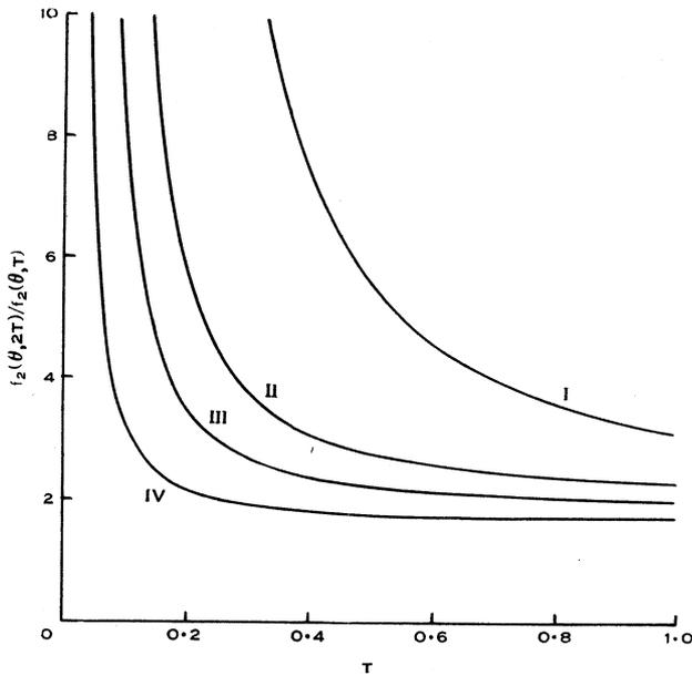
Fig. 6.—Values of  $f_2(\theta, 2T)/f_2(\theta, T)$ . Curves I, II, III, IV are for  $\theta=180, 90, 69, 45^\circ$  respectively.
