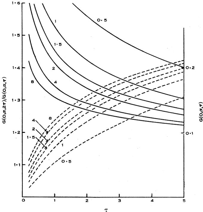
Fig. 7.—Values of  $G(0, \alpha, \tau)$ : dotted lines, right-hand scale. Values of  $G(0, \alpha, 2\tau)/G(0, \alpha, \tau)$ : full lines, left-hand scale. The numbers on the curves are the values of  $\alpha$ .
