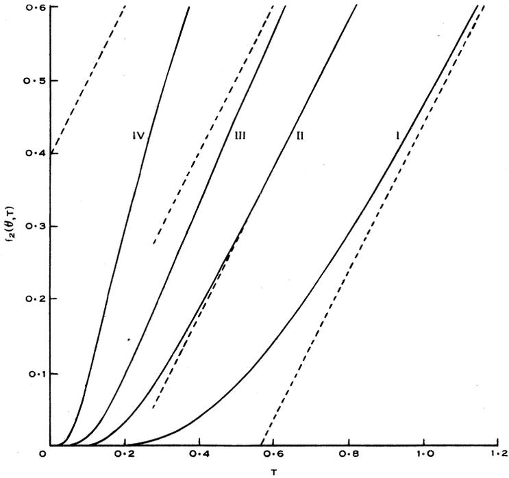
Fig. 5.—Values of  $f_2(\theta, T)$ . Curves I, II, III, IV are for  $\theta=180, 90, 69, 45^\circ$  respectively. The asymptotes are shown by dotted lines.
