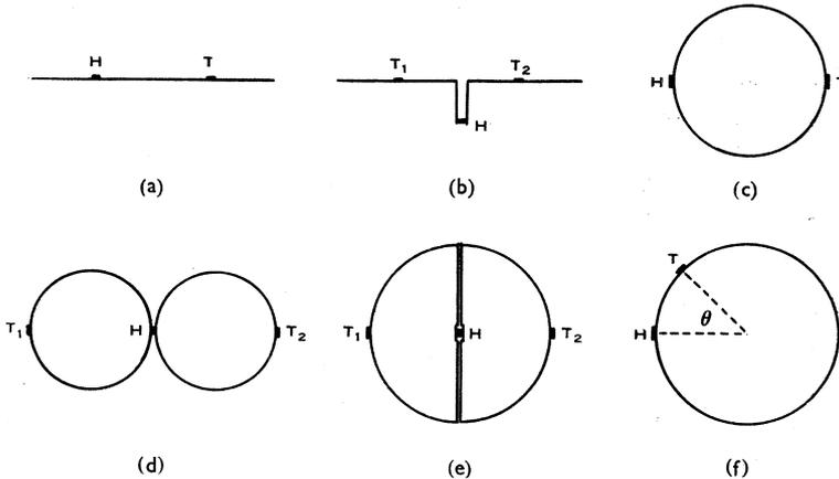
Fig. 1.—Cross sections of some possible systems for the determination of the thermal conductivity of rock specimens. *H*, heater wire; *T*, *T*<sub>1</sub>, *T*<sub>2</sub>, thermocouples.
