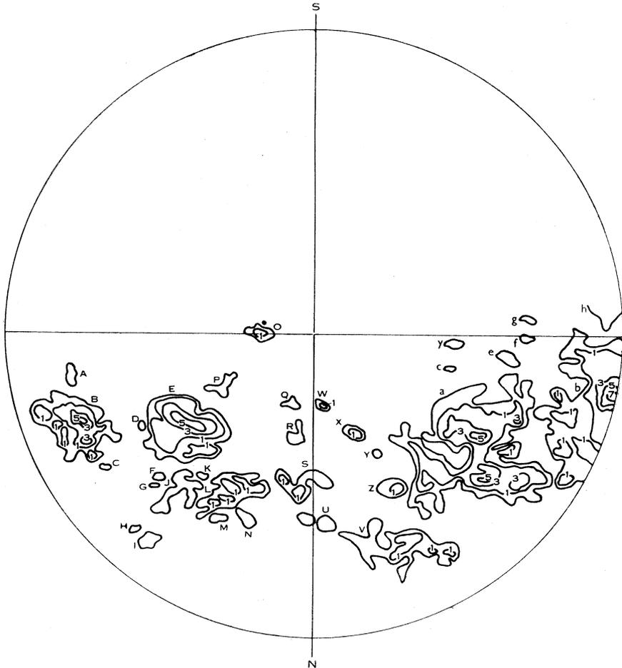
Fig. 5.—The distribution of optical plages as seen in the *K* line of calcium is shown. This was obtained by photometering the distribution shown in Plate 1 and compensating for the rotation of the Sun between the taking of Plate 1 and the time of the eclipse. The contour intervals are those described in Section IV (a). The outermost contours are not numbered and the letters attached to each region are used to label them for discussion.
