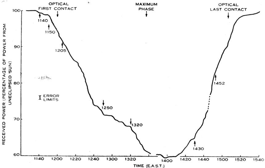
Fig. 3.—The power received by the radiometer from the Sun during the eclipse is shown. The curve was obtained by taking values at intervals of 1 min from the output record of the radiometer. The dashed region corresponds to an interval of 2 min when calibrations were made. The arrows show the various times of interest in Section IV.
