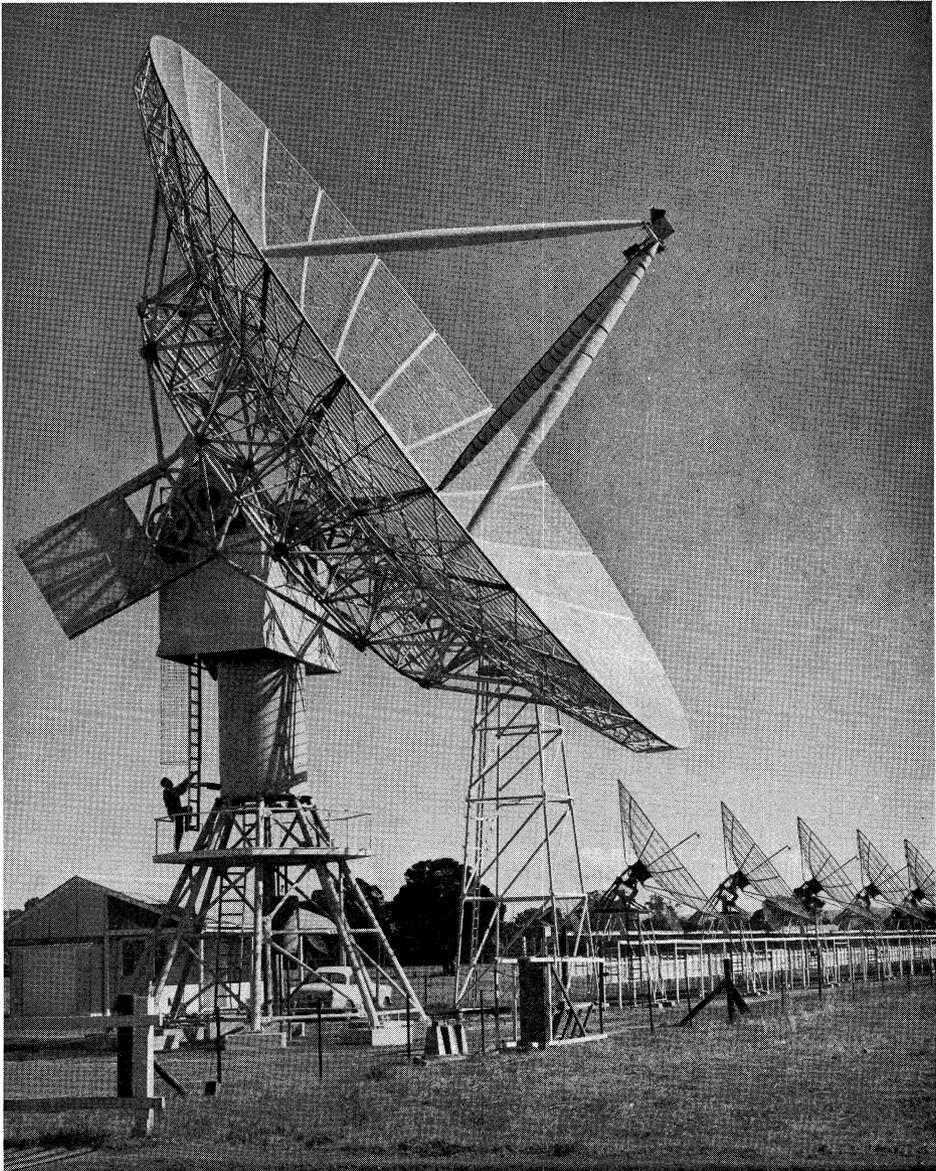
The 60-ft Kennedy paraboloid at Fleurs Field Station, with the 18-ft paraboloids of the crossed multiple interferometer (Christiansen and Mathewson 1958) in the background.
