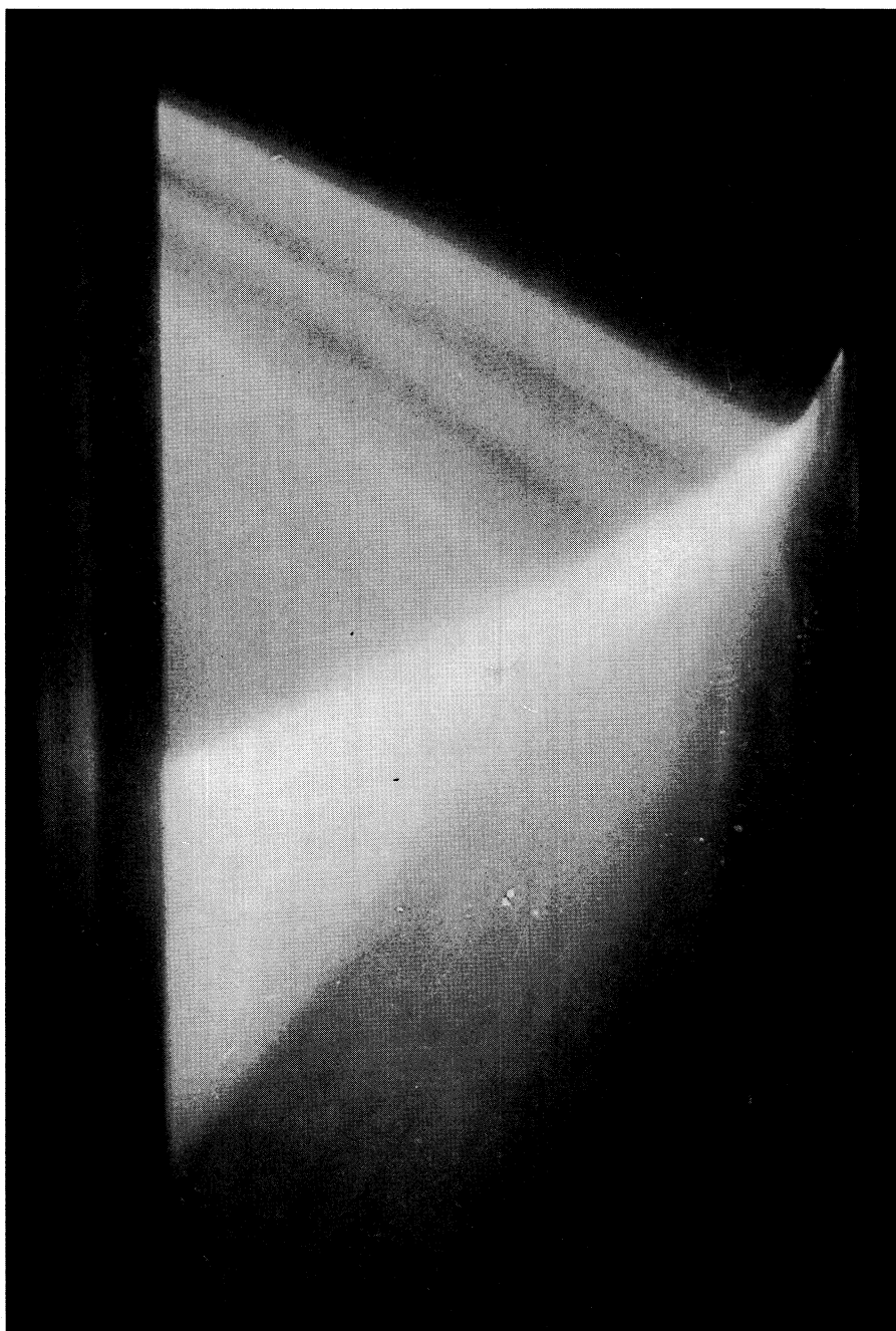
Fig. 6.—Single x-t streak record of a shock in air at 5 torr initial pressure that is reflected from a ceramic end wall 20 cm from the ring electrode.
