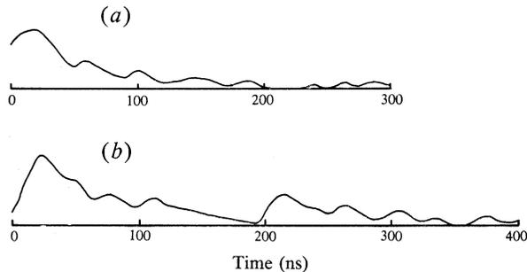
**Fig. 4.** Two observed pulses for (a) an analysed shower a little more than 200 m from the core (pulse area corresponds to 1.1 vertical equivalent muons); (b) a large shower at a large distance ( $\geq 250$  m) from the core. No detailed array analysis is available for the second event which had a large zenith angle ( $46^\circ$ ) (pulse area corresponds to 1.7 vertical equivalent muons).
