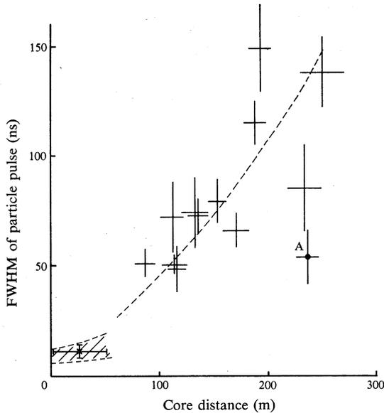
**Fig. 3.** Measured relationship between shower core distance and the FWHM of the particle pulse. The FWHM of the system was 36 ns. The dashed curve indicates the dispersion ( $2\times$ ) given by Linsley as a rough approximation to the expected function. The data marked by a cross (at lower left) are undeconvolved results of McDonald *et al.* (1977). The hatched area is from Sakuyama and Suzuki (1981).
