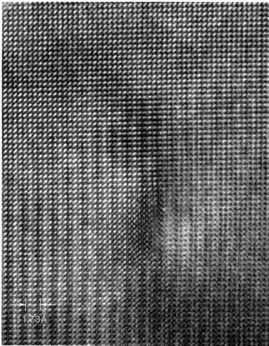
**Fig. 1.** Lattice image of a dislocation including slowly varying contrast due to strain. Contrast reversal in the lattice image due to the tilt induced by the strain field of the dislocation is evident.
