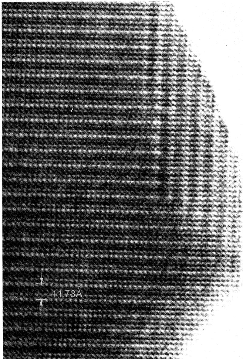
Fig. 6. Lattice image of naturally grown facets in  $\text{La}_3\text{Ba}_3\text{Cu}_6\text{O}_{14}$ . Contrast due to surface steps is superimposed on the lattice images. Steps can also be seen in profile.
