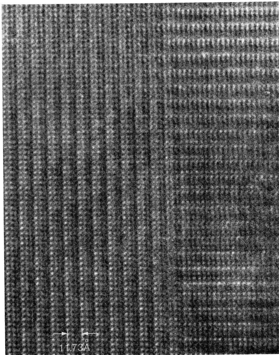
**Fig. 2.** Lattice image of an interface in  $\text{La}_3\text{Ba}_3\text{Cu}_6\text{O}_{14}$ . The plane of projection is (100) in each crystal and the  $c$  axes are orthogonal. No strain or tilt can be detected in this one-dimensional intergrowth.
