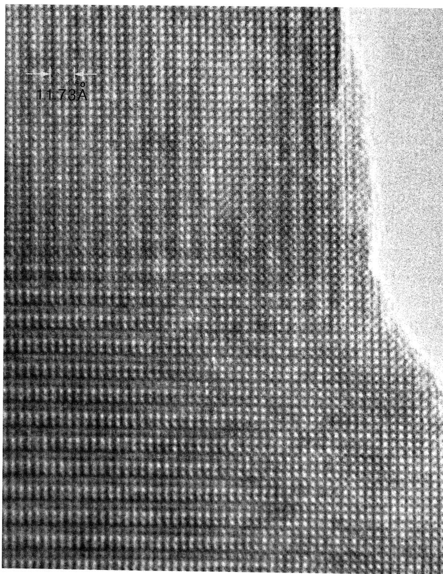
Fig. 3. Lattice image of two-dimensional overgrowth in  $\text{La}_3\text{Ba}_3\text{Cu}_6\text{O}_{14}$ .
