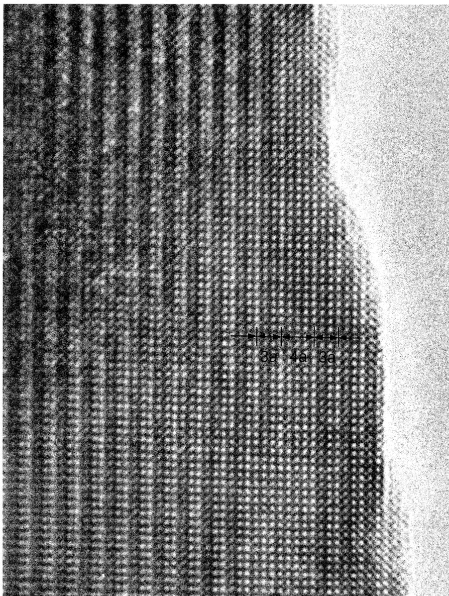
Fig. 5. Lattice image of  $\text{La}_3\text{Ba}_3\text{Cu}_6\text{O}_{14}$  showing intergrowth of a plate of crystal with  $c/a = 4$ .
