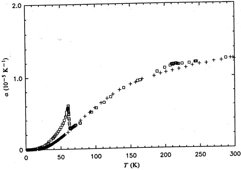
Fig. 4. Squares: linear thermal expansion coefficient data; crosses: non-magnetic background for  $\text{Fe}_2\text{MnSi}$  as a function of temperature.
