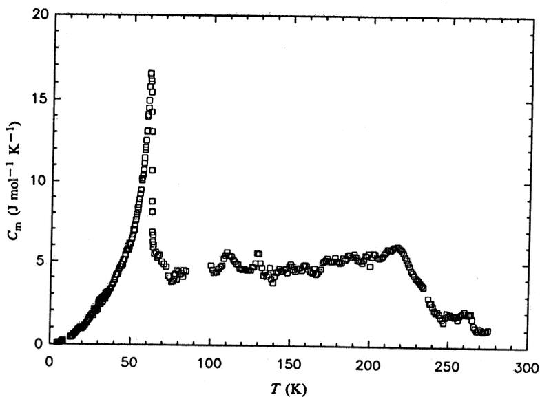
Fig. 3. Magnetic contribution to the specific heat for  $\text{Fe}_2\text{MnSi}$ .
