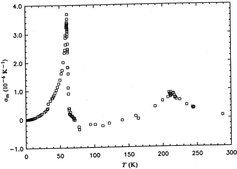
Fig. 5. Magnetic contribution to the linear thermal expansion coefficient of  $\text{Fe}_2\text{MnSi}$  as a function of temperature.
