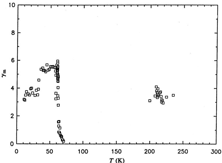
Fig. 6. Magnetic Grüneisen parameter for Fe<sub>2</sub>MnSi as a function of temperature.
