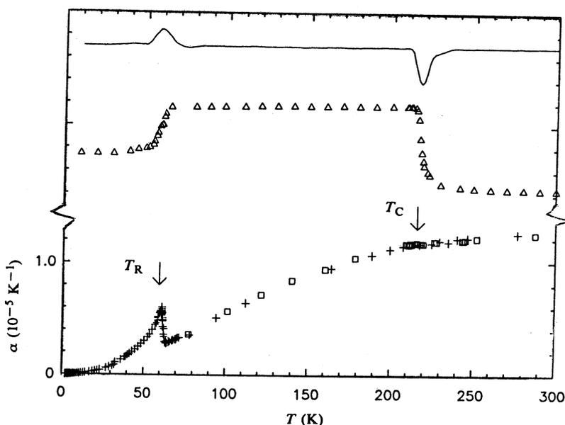
Fig. 1. Linear thermal expansion for  $\text{Fe}_2\text{MnSi}$  as a function of temperature: Pluses, quenched sample; squares, slow-cooled sample; triangles, secondary coil signal (arbitrary units); and solid curve, derivative of the interpolated coil signal.
