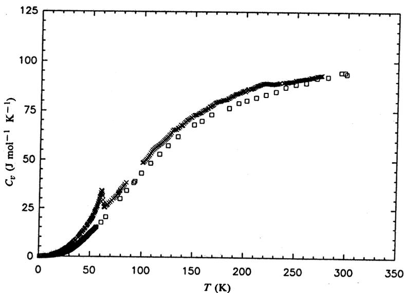
Fig. 2. Specific heat data: Crosses,  $\text{Fe}_2\text{MnSi}$ ; squares,  $\text{Fe}_3\text{Si}$ .
