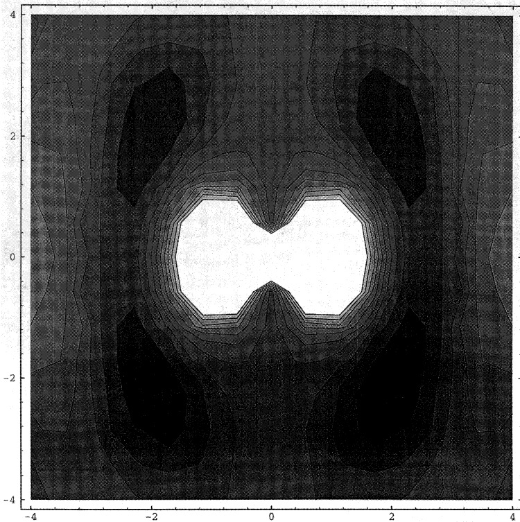
Fig. 6. Energy portrait for the case of magnetic polarisation and scalar interaction (case B in the text). The singularity for r = 0 is absent (see equation 20).
