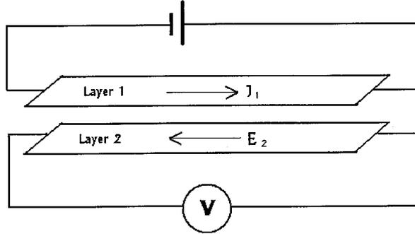
**Fig. 1.** Schematic diagram of a frictional drag experiment in a coupled 2DEG. A current  $\mathbf{J}_1$  is passed through layer 1, and the interlayer interaction induces a transfer of momentum to the carriers in layer 2, dragging these carriers along. In the steady state, charges in layer 2 pile up on one side of the sample, producing an electric field  $\mathbf{E}_2$  which negates the drag force. This electric field can be measured experimentally.
