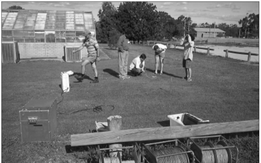
Top: Margaret Ang (Monash University) and Matt Bull (University of Adelaide) conduct a resistivity survey using a Geometrics TR1 OhmMAPPER, a capacitively coupled device. Dookie, November 2001.
