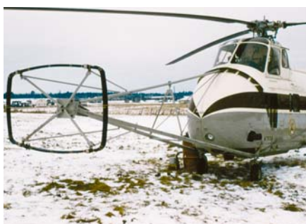
Fig. 5. Transmitter coil on Newmont Aero Service EM system mounted on a Sikorsky S-55 helicopter ~1956.
