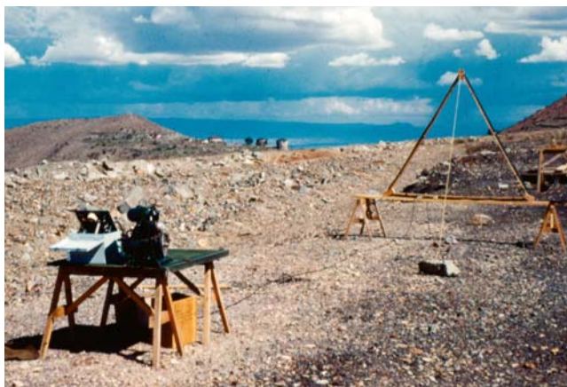
Fig. 6. Early EM tests at Jerome, Arizona ~1955. The triangle shaped transmitter coil was a prototype for the airborne EM system.
