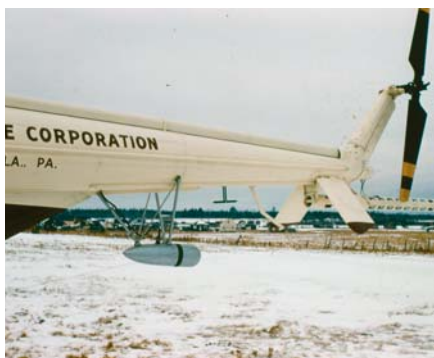
Fig. 4. Magnetometer and EM receiver coil on Newmont Aero Service frequency-domain EM system ~1956.
