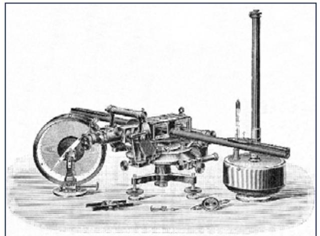
Fig. 5. A dip circle, declinometer/magnetometer and torsion compass; G. von Neumayer and J. Edler circa 1903.
