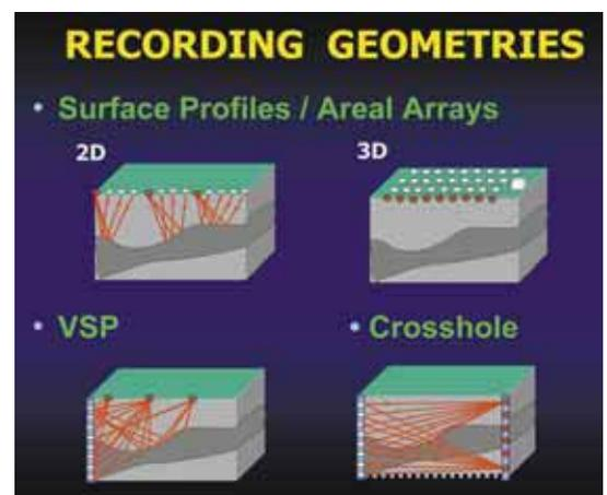
Fig. 1. Various recording geometries for seismic surveying - surface (2D or 3D), VSP and cross-hole. Source and receiver points are placed on the Earth's surface (linear or aerial arrays) and/or down boreholes.
