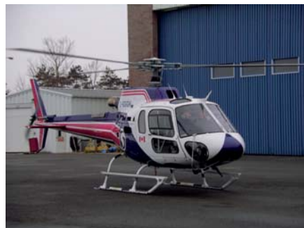
Fig. 1. Feynman Eurocopter AS350-B3 Helicopter Platform. The platform allows collection of gravity, magnetics, laser-scanner DEM and electromagnetic datasets simultaneously.
