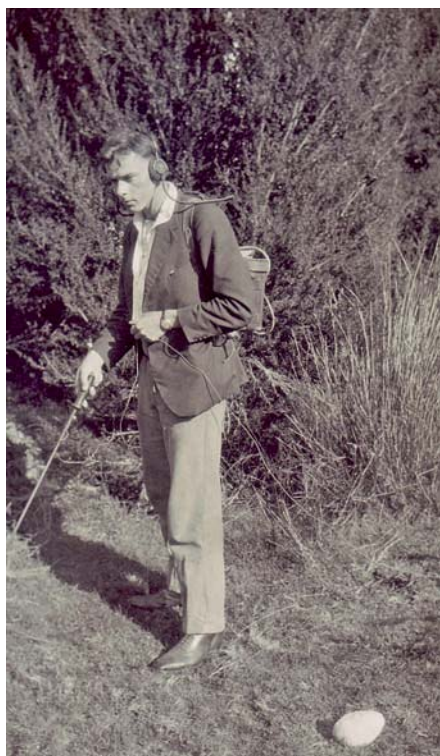
Fig. 8. Jack mapping equipotentials, west coast of Tasmania about 1929: rapier in hand, amplifier on his back and polished shoes ready for the bush.
