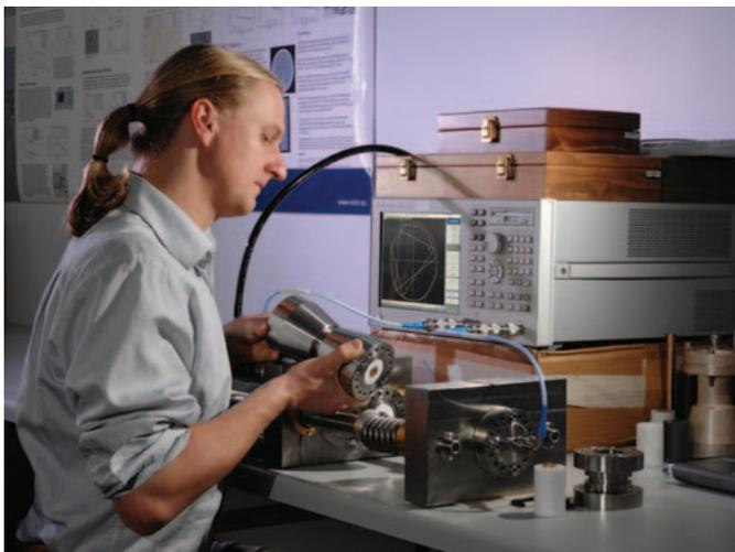
Dielectric rock testing at CSIRO laboratories.
