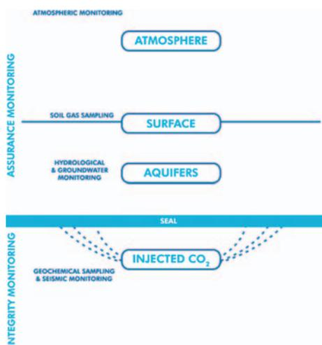
Schematic of the various elements of CO<sub>2</sub> monitoring.
