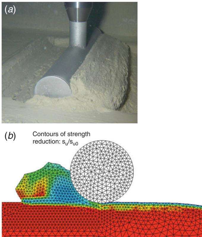
**Fig. 2.** Physical and numerical modelling of pipeline-seabed interaction. (a) Geotechnical centrifuge modelling (Gaudin and White 2009). (b) Large deformation finite element analysis (Wang et al. 2010).
