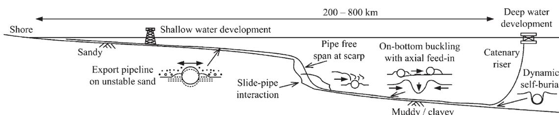
Fig. 1. Changing infrastructure as hydrocarbon developments move into deeper water.
