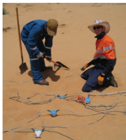
Fig. 2. Burying the UniQ geophone accelerometers.
