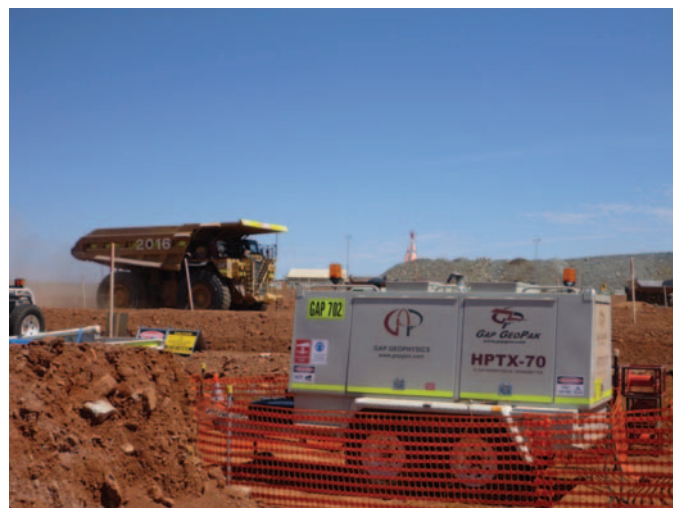
Fig. 1. The HPTX-70 high-powered geophysical transmitter.
