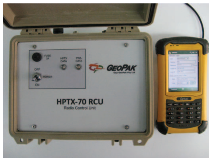
Fig. 9. The HPTX-70 control system includes a ruggedised handheld computer and radio modem.
