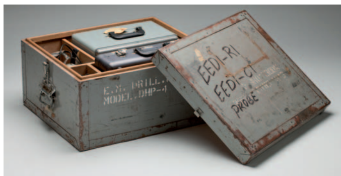
Fig. 8. Scintrex DHP-4 electromagnetic drill-hole probe. Image: National Museum of Australia.
