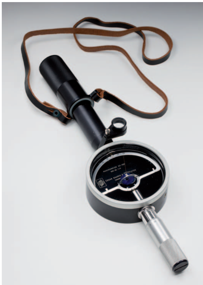
Fig. 3. Sharp personal torsion magnetometer. Image: National Museum of Australia.
