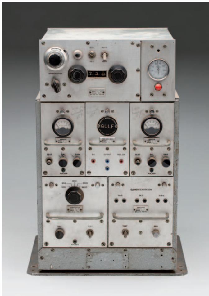
Fig. 4. Hunting Adastra Gulf airborne magnetometer. Image: Denis Shephard, 2012.
