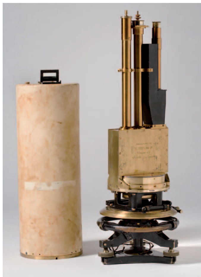
Fig. 2. Oertling gradiometer no. 21636, dating 1928. Implementation: Used on the Imperial Geophysical Experimental Survey. Image: National Museum of Australia, 2006.
