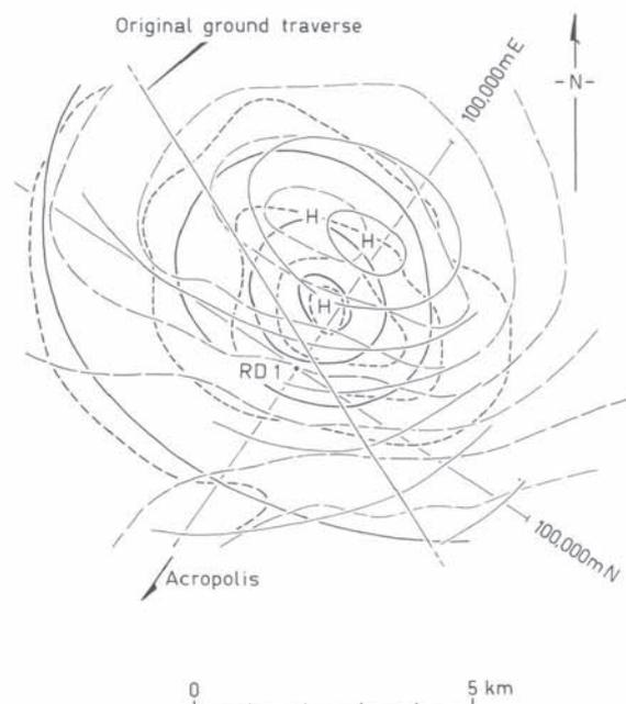
Fig 5 Geophysical summary. Magnetic contours: — original; - - detail. Gravity contours: — original; --- detail.
