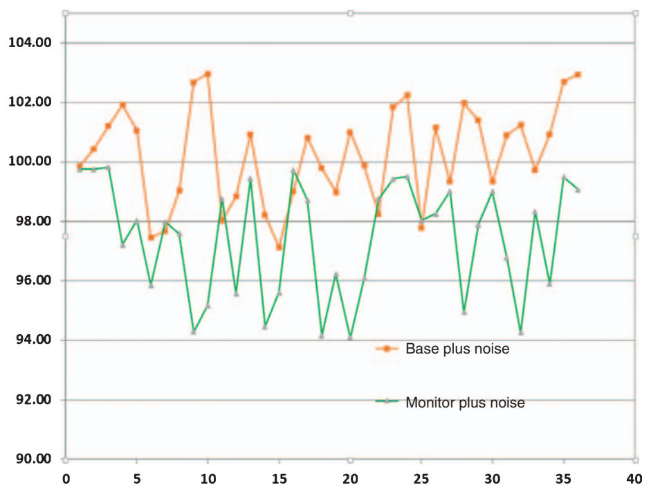
Figure 2. Modelled amplitude of base survey and monitor survey in the presence of different random noise for each. Vertical axis is amplitude, horizontal axis represents CDP location. Original amplitudes are 100 for base and 97 for monitor which represents a 3% change. There is significant overlap between the two lines.
