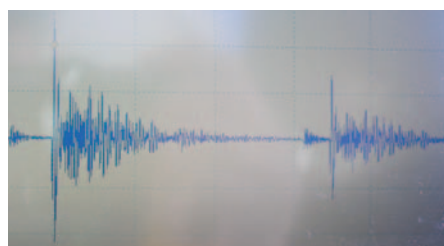
Figure 2. Photograph of typical ice radar return. In this image, each vertical increment represents 40 mV and each horizontal increment 1.0 \mu s. The yellow diamond shows the value (+80 mV) at which the oscilloscope trigger was set to commence data capture.
