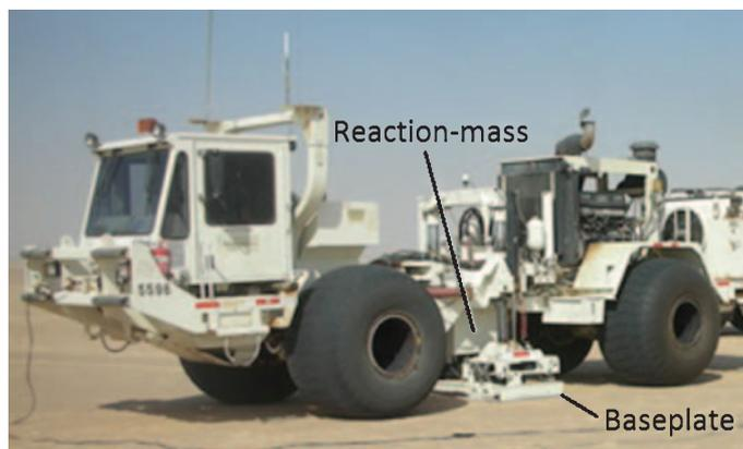
**Figure 1.** A hydraulic vibrator in action. The baseplate is on the ground between the two axles. The reaction-mass is the large white steel cube directly above the baseplate.
