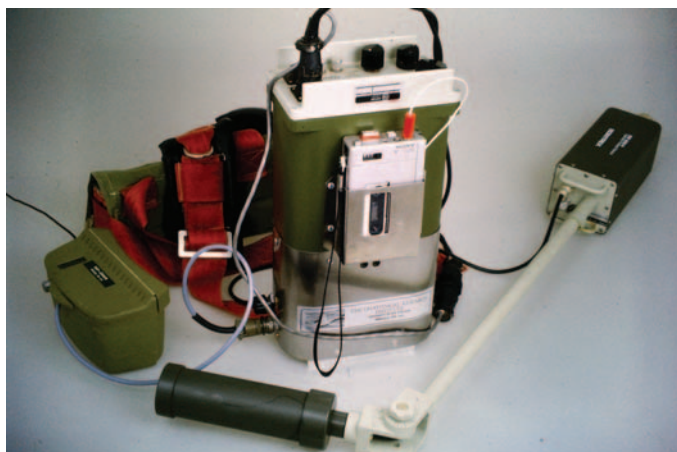
Figure 7. In 1980 the TM-1 prototype was upgraded using facilities available in the Varian sensor controller/frequency counter module. Digital data and voice notes were recorded in real time at sample intervals automatically determined by a cotton thread type odometer. Positioned measurements at sub-metre intervals could be acquired at survey speeds faster than the operator could walk.
