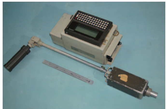
Figure 11. The TM-3 magnetometer with microprocessor controlled survey management aids, inbuilt odometer and digital recording from up to two optically pumped sensors.
