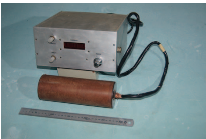
Figure 2. The first 'digital alkali vapour magnetometer using integrated circuits'. The release of TTL digital logic integrated circuit devices permitted a magnetometer to be built in 1973 that took the Larmor signal from an optically pumped sensor, and from this determine a digital measure of the Total Magnetic Intensity. A 1 nT resolution could be updated approximately 45 times per second.
