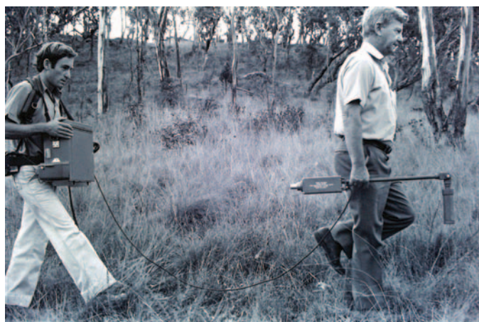
Figure 6. The 'telemetric magnetometer' TM-1 encoded digital data in an audio code suitable for transmitting by CB radio to the vehicle-borne digital data acquisition system. With the advent of the Sony Walkman cassette recorder in 1979, the troublesome CB link was replaced. The instrument shown here was the first portable magnetometer with inbuilt memory and a data positioning device.
