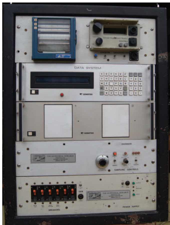
Figure 5. With the advent of the microprocessor, a digital data logging and replay facility was added to a vehicle mounted survey system. Data acquisition programs and data logging were now interfaced with a digital cassette tape recorder.
