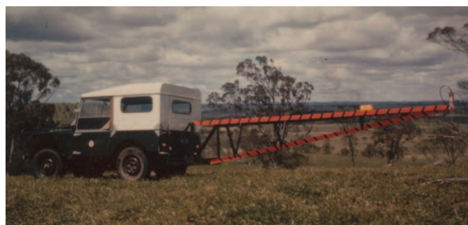
Figure 4. The vehicle-borne magnetometer in which the Cs magnetometer sensor was mounted in a plane where the contour line of interference from the vehicle's magnetic field was almost circular. The result was a heading error of just 0.07 nT per degree. Magnetic data were automatically logged to scale on a chart recorder triggered from the vehicle odometer. Measurements were acquired at 0.25 m intervals while travelling.
