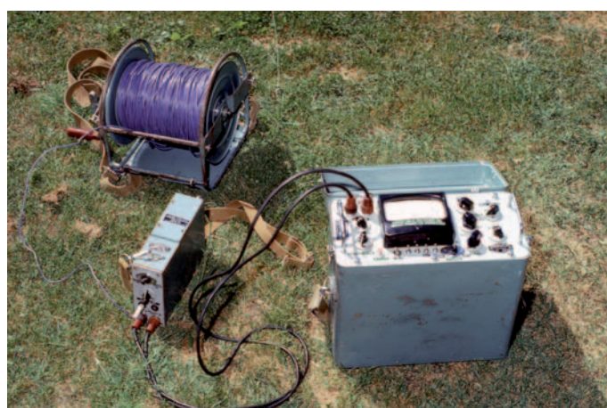
Figure 2. MPPO-1 transmitter pack (lower left) and receiver unit (right). The main settings on the receiver are selection of transient decay time (bottom left) ranging from 1 ms to 15 ms, amplification (mid-right), and two settings of noise damping (bottom right). The transmitter sends 20-ms wide rectangular pulses at the rate of 18 Hz into the combined transmitter/receiver loop.
