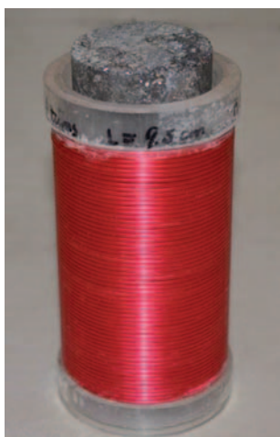
Figure 2. This photograph shows an induction coil of the type used in the measurements. It is 95 mm long x 50 mm internal diameter; the cylindrical housing is 120 mm long. At a particular frequency (below the onset of the skin effect) the change in resistance ( \Delta R ) and in inductance ( \Delta L ) are measured on an impedance bridge when a core is inserted. From these quantities, conductivity ( \Delta R ) and magnetic susceptibility ( \Delta L ) are calculated (see Yang and Emerson, 1997).
