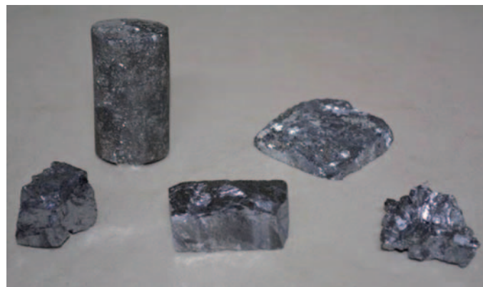
Figure 1. This photograph shows subsamples representative of some of the cored galena materials. The first prism, on the left, is from Sweetwater, Missouri; it has 10 mm \pm grainsize and an EM conductivity of 7812 S/m. The second prism, in the middle, is from Rapid Bay South Australia; it has 5 mm \pm grainsize and conductivity of 6364 S/m. These two prisms are virtually pure galena continua. The third subsample of irregular outline on the right is from Dalnegorsk in Russia; it has 5 mm \pm grainsize but it contains some gangue, voids, and other discontinuities so its lower conductivity of 3010 S/m is not unexpected. The slab is from the parent lead lode material from which L10 was cored (see Table 1), it contains about 60% by volume of distributed galena with grainsize 2 mm \pm ; L10’s conductivity is 587 S/m. The 45 mm diameter core is Z3 from the zinc lode suite with 70% marmatite, 15% galena, and small percentages of pyrrhotite/chalcopyrite that have contributed to Z3’s conductivity of 87 S/m. In the photo the galena, or at least some of it, can be identified by the metallic reflections, but the wispy pyrrhotite and chalcopyrite in Z3 cannot be seen at this scale.
