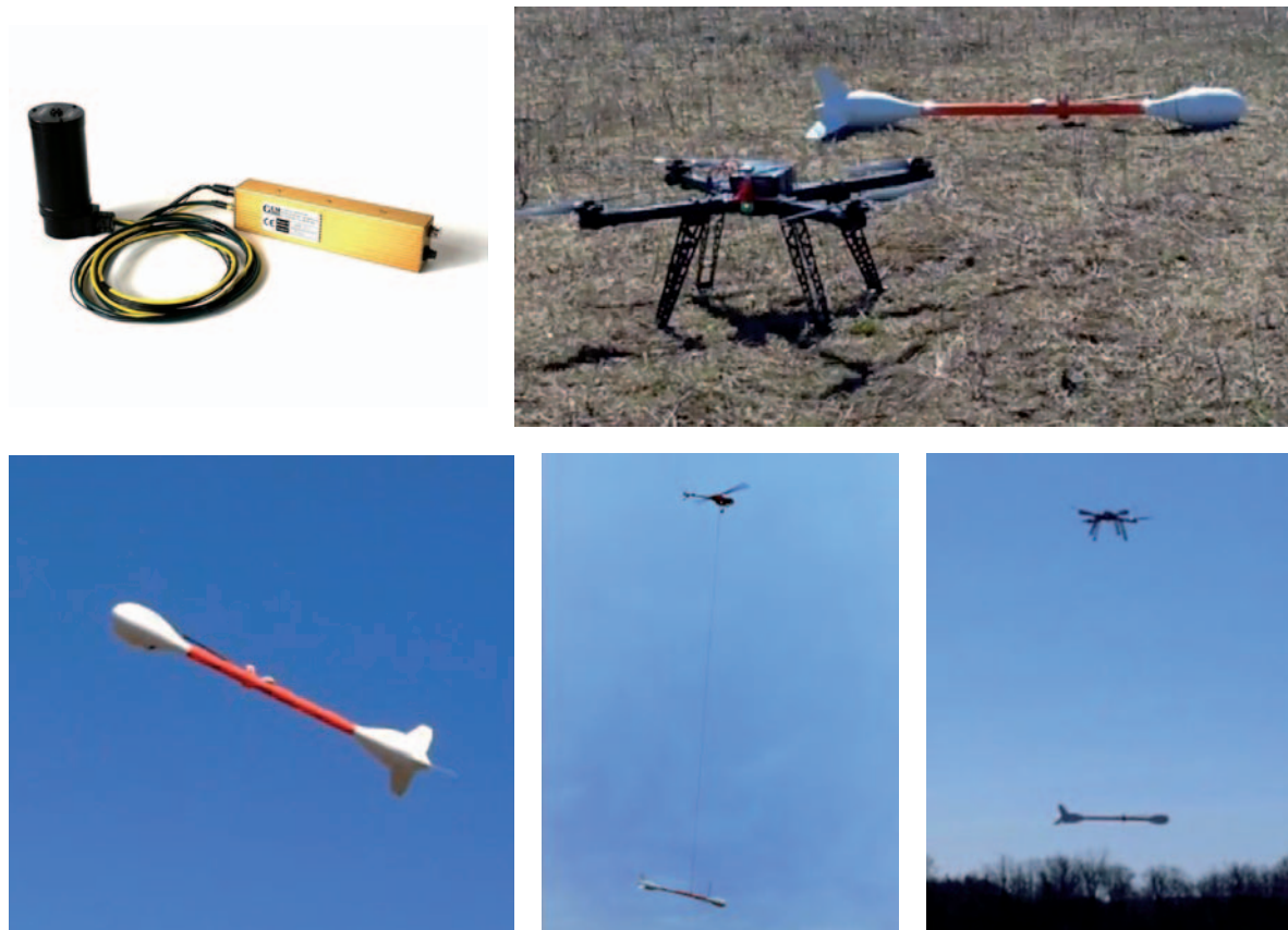
Figure 1. Sling-mounted magnetometer weighing ~3.3 kg hanging under various UAVs. The system's heart is the Gem GSMP 35U Potassium UAV magnetometer shown in the upper left ( www.gemsys.ca/uavs-pathway-to-the-future/ ).
