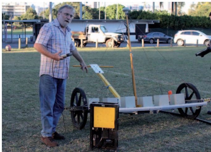
Stephen Griffin of Gap Geophysics explains the features of the UltraTEM2 precision UXO and metal-detection cart.
