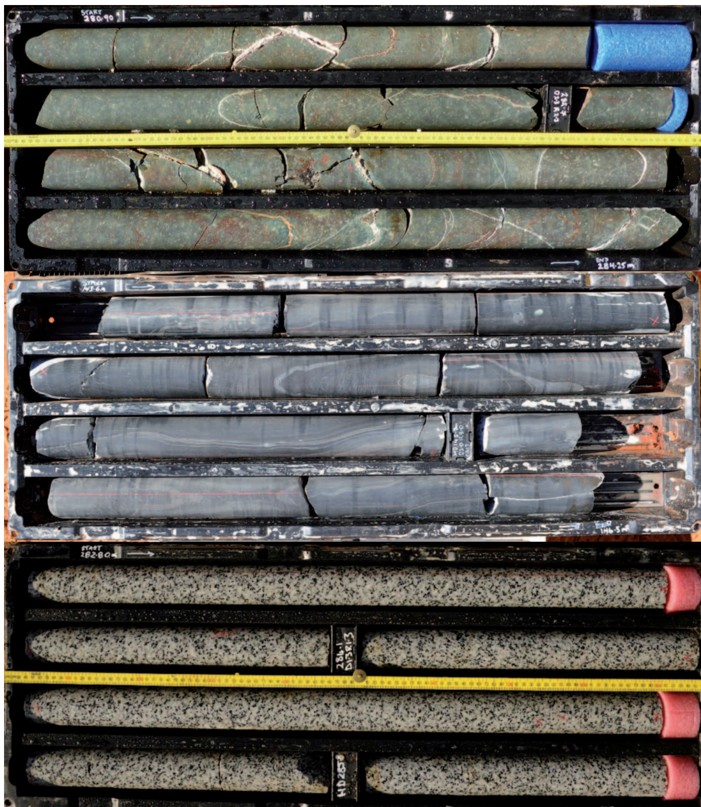
Figure 2. Rhyodacite core from GSNW Milcarpa 1 (top), metasedimentary schist from GSNW Euroli 1 (centre) and granodiorite from GSNW Tongo 1 (below).
