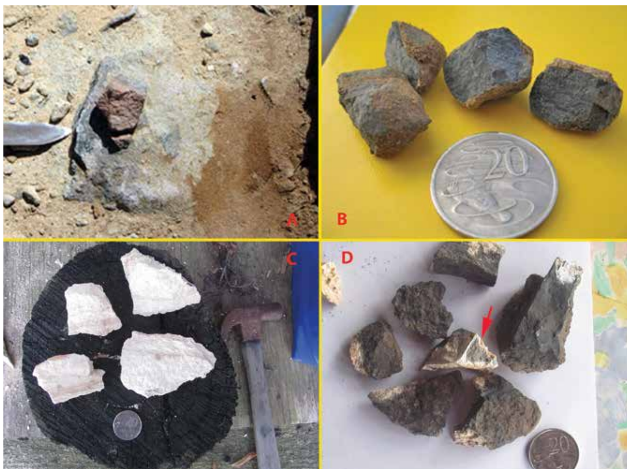
Figure 18: Experimental fire conversion to dark calcrete.
