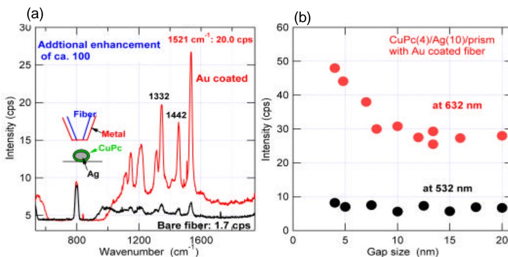
Fig. 2 Tip enhanced near-field Raman spectra from CuPc(1.5nm)/Ag(5 nm)/prism: (a) effect of metal coating to the fiber, (b) gap size dependence of the signal intensity. Metal coating to the fiber probe increases the Raman signal by ca.100 at smaller gap sizes (b).
