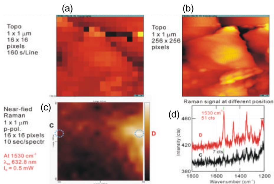
Fig. 1 Topography (a, b), near-field Raman image (c) and spectra (d) from CuPc(1.5nm)/Ag(5 nm)/prism using an etched optical fiber probe. The topography (b) with sufficiently high resolution (256×256) was obtained at first, then with lower resolution (16×16 pixels) topography and SERS spectra (d) were observed with 10 s for accumulation. After the measurement, Raman peak intensity at 1530 cm<sup>-1</sup> was evaluated at each position to reconstruct the near-field Raman image as in (c).
