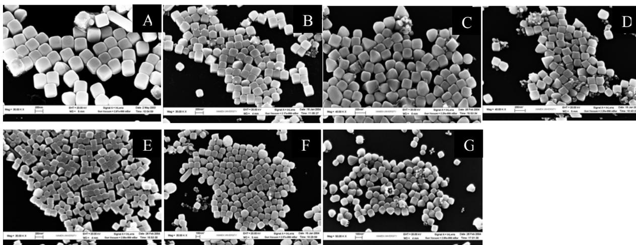
Fig.1. SEM images of silver nanocubes with various sizes on silicon wafers. The edge length of silver nanocubes are: (A) 330 nm, (B) 200 nm, (C) 175 nm, (D) 150 nm, (E) 136 nm, (F) 126 nm, (G) 84 nm.
