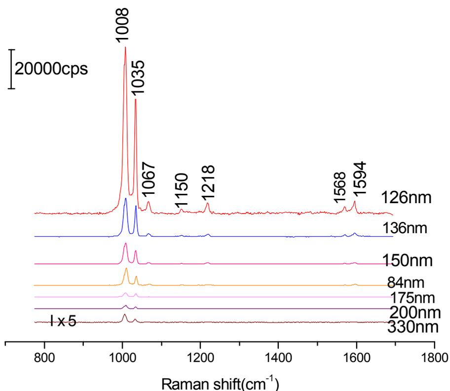
Fig.2. SERS spectra of pyridine (0.01 M) from silver nanocubes with various sizes assembled on silicon wafers. Excitation line: 632.8 nm
