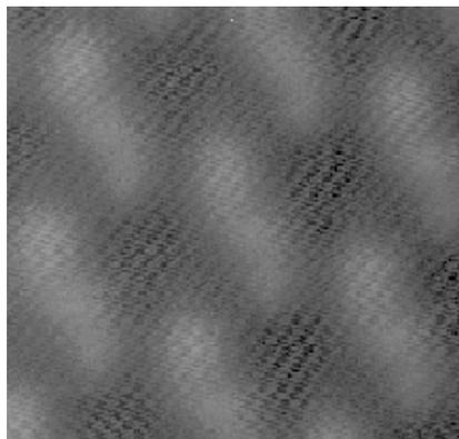
**Fig. 2.** STM image of a 2D array of PS II core complexes (image size, 60 x 60 nm).
