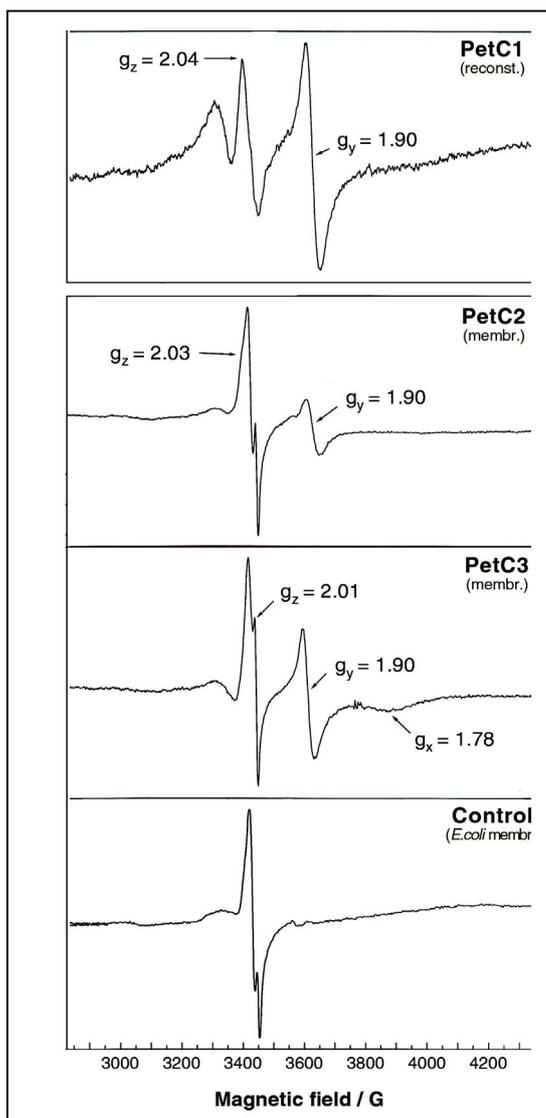
**Fig. 3.** EPR spectra of *Synechocystis* Rieske proteins after purification and reconstitution (PetC1) or of *E. coli* membranes with incorporated PetC2 and PetC3 and of control membranes recorded at 15 K.
