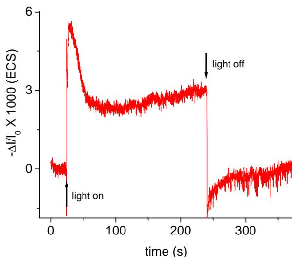
**Figure 2.** Absorbance changes attributable to ECS in an intact, *npq4* mutant *Arabidopsis* leaf. The actinic light ( $1200 \mu\text{E m}^{-2} \text{s}^{-1}$  red light) was activated at the up arrow and deactivated at the down arrow. Absorbance data was collected at 4 wavelengths simultaneously (505, 525 nm, 535 nm and 545 nm) at intervals of 4 ms and the trace was deconvoluted as described in (Cruz et al, 2000)
